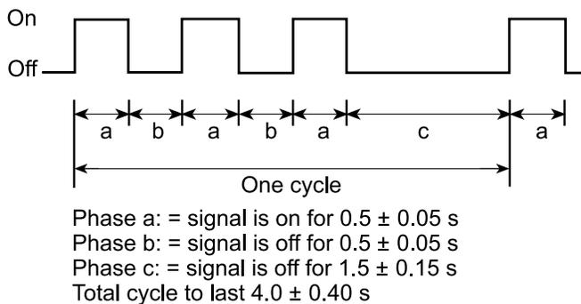
Figure 2. Temporal-Three pattern for fire evacuation alarm signal
