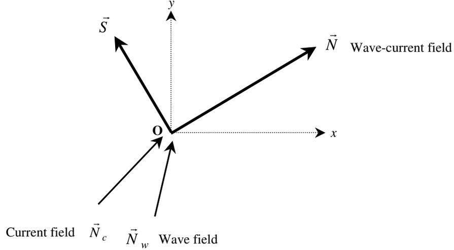
Fig.1 Wave-free current, current-free wave and wave-current fields relative directions
