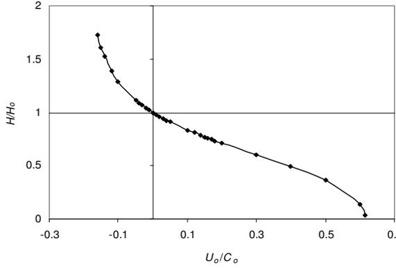
Fig. 6 Variation of wave height  $H/H_0$  with  $U_0/C_0$
