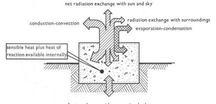
heat exchange with connecting body
