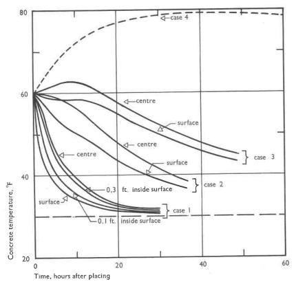
RILEM 56 A l.dlo: Fig.12. Temperature in a One-foot Thick Concrete Wall Exposed on Both Sides (initial placing temperature 60  $^{\circ}$ F.; air temperature 30  $^{\circ}$ F.).
