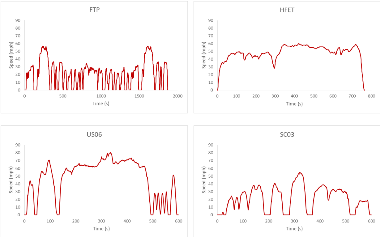
Figure 2: Drive cycles for EPA dynamometer tests: a) FTP test for city driving, b) HFET test for highway driving, c) US06 test for aggressive driving, d) SC03 test for air conditioning.
