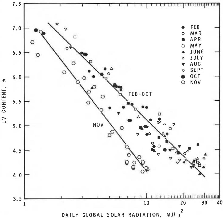
Fig. 6. Percent UV radiation vs. daily total (global) solar radiation on horizontal surface, February—November 1981.
