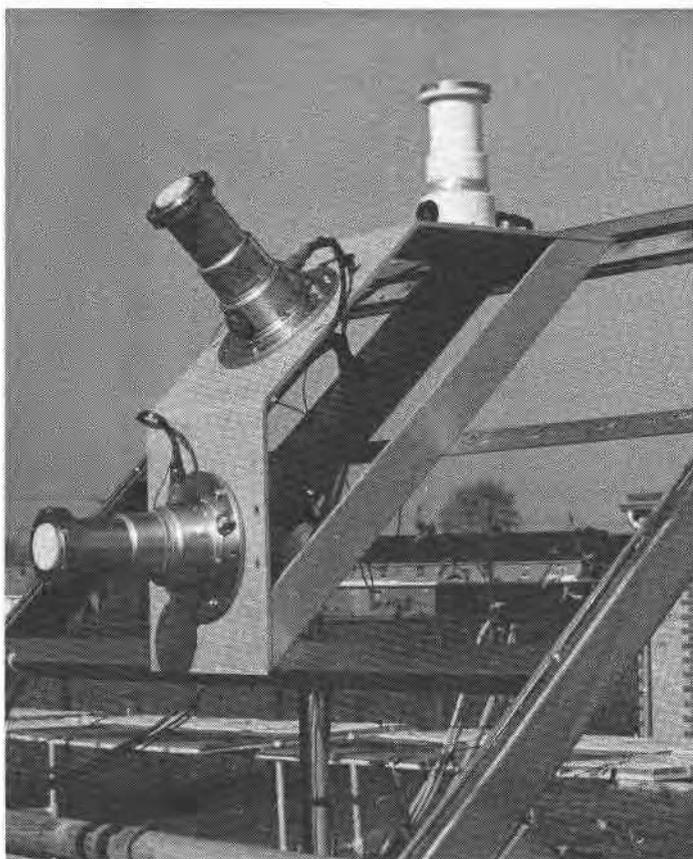
Fig. 1. Apparatus for measuring solar UV radiation incident on H, S/45 and S/V surfaces.
