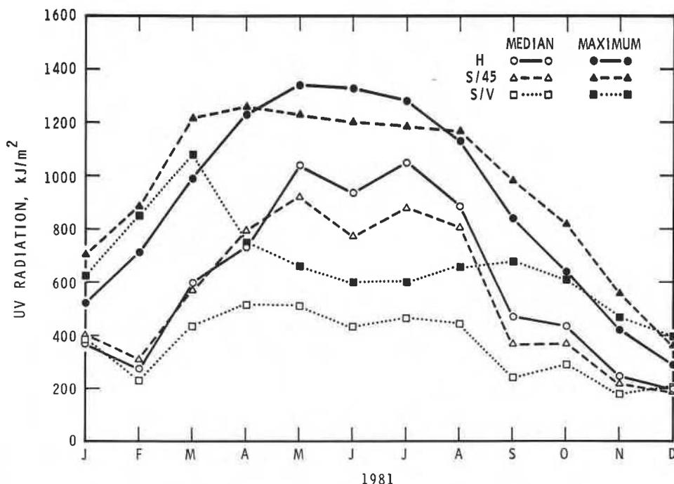
Fig. 4. Level and variation of median and maximum daily UV radiation on surfaces, monthly basis.
