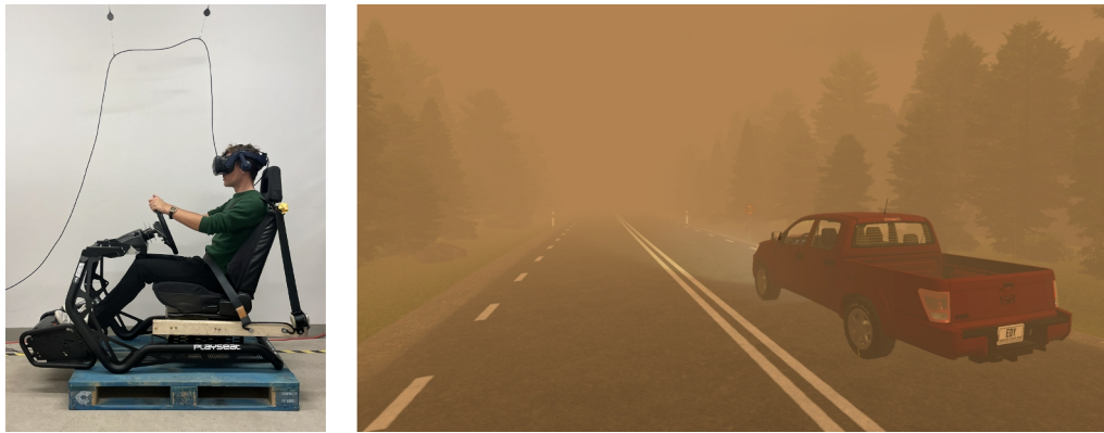
Fig. 1. Left: the hardware used for interaction with the virtual environment. Right: the virtual road and the virtual vehicle controlled by the participant. In this figure, the extinction factor K equals 0.05 \text{ m}^{-1} .
