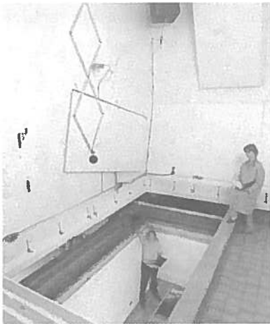
IRC's full-scale facility for acoustical testing of floor assemblies
