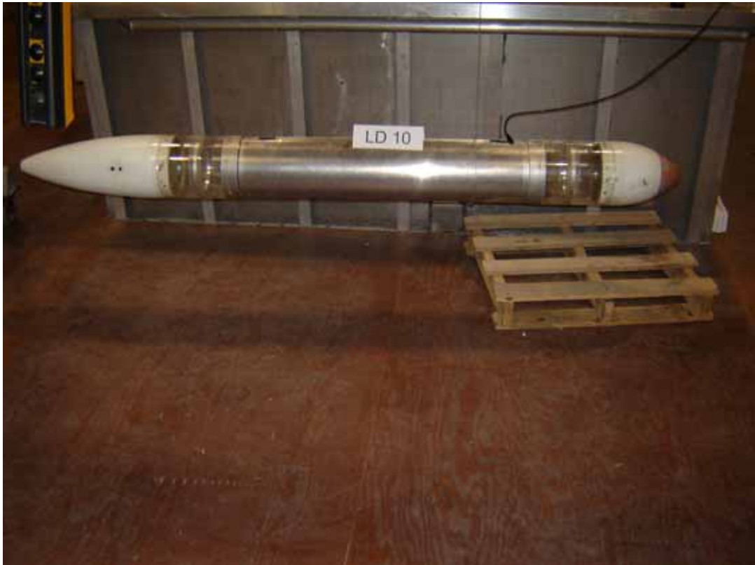
Figure 6 - LD 10 hanging for dry swing tests
