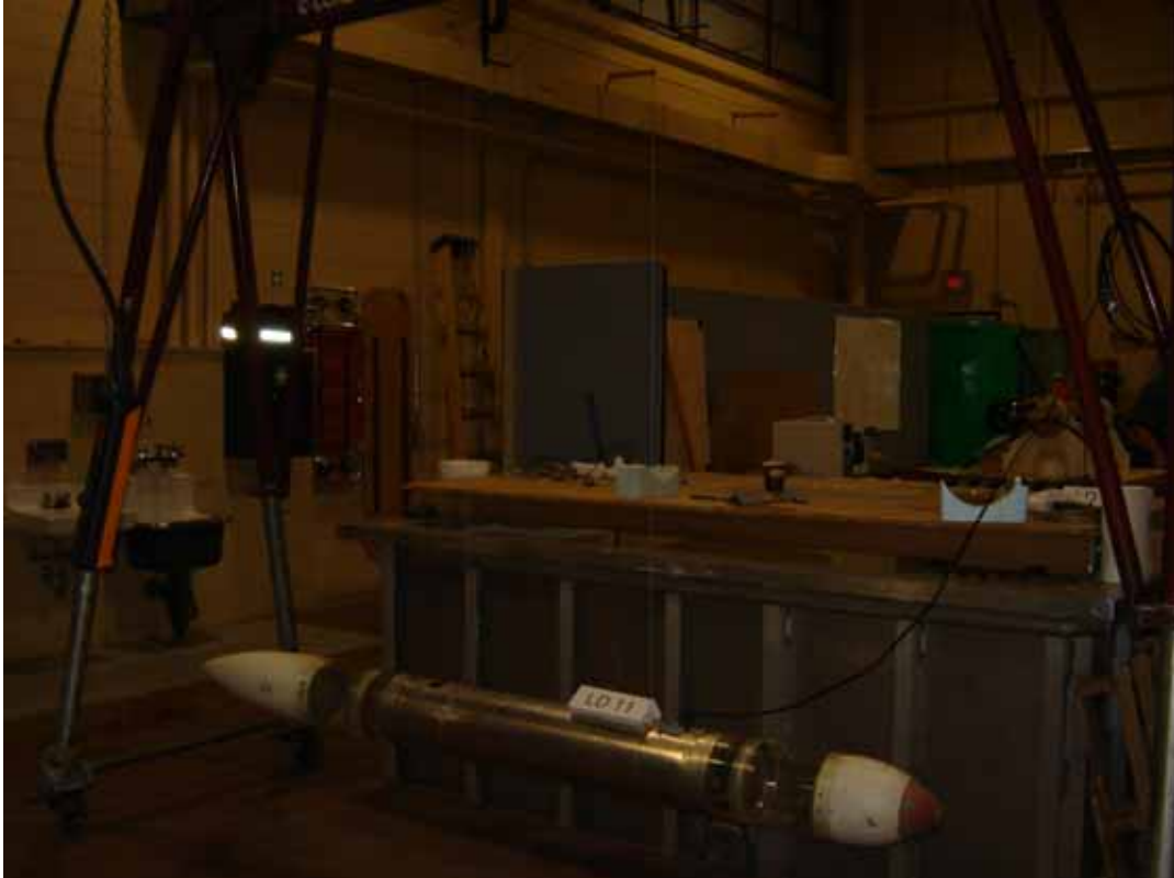
Figure 8 - LD 11 hanging for dry swing tests
