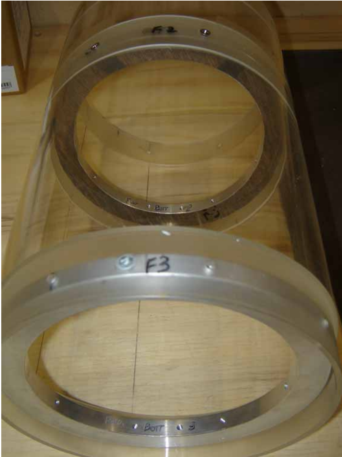
Figure 3 - Connection of two adjacent acrylic pieces
