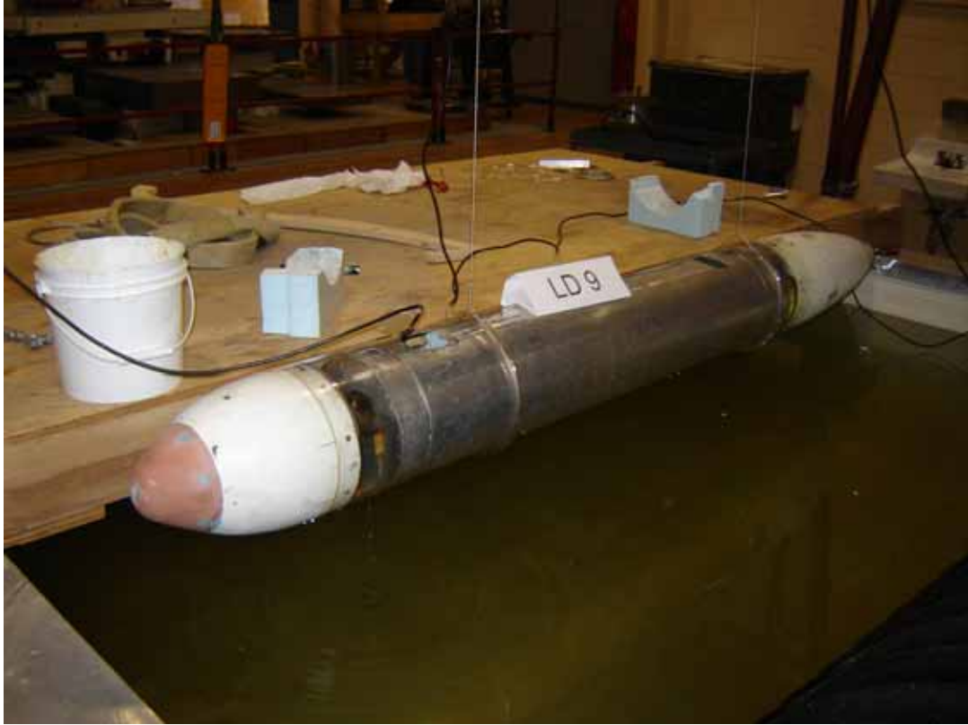
Figure 5 - LD 9 flooded for wet swing tests
