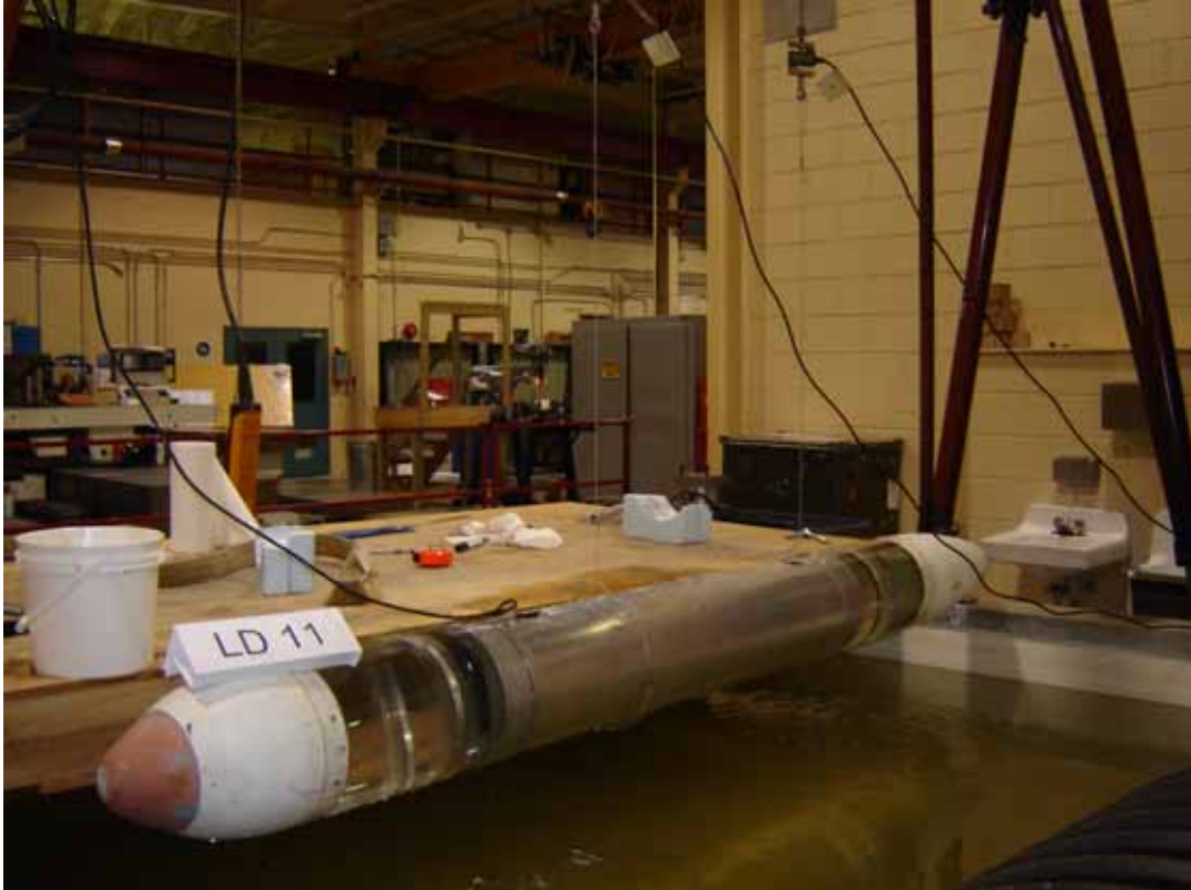
Figure 10 - LD 11 flooded for wet swing tests
