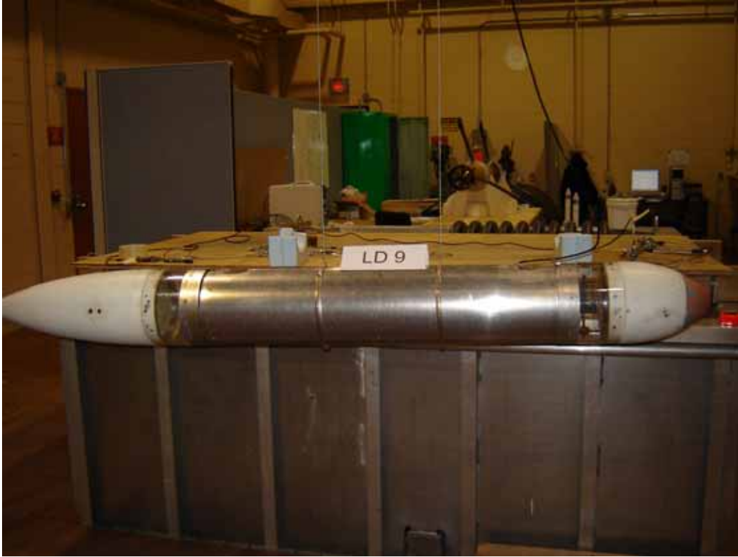
Figure 3 - LD 9 hanging for dry swing tests
