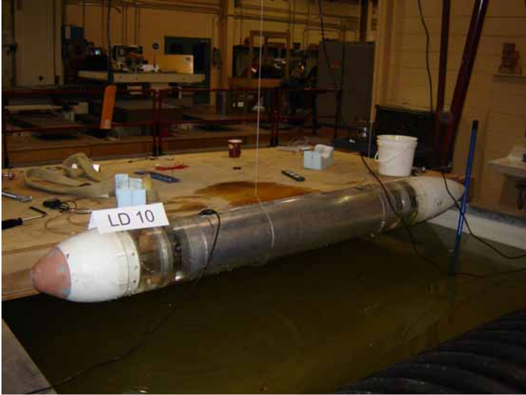
Figure 7 - LD 10 flooded for wet swing tests
