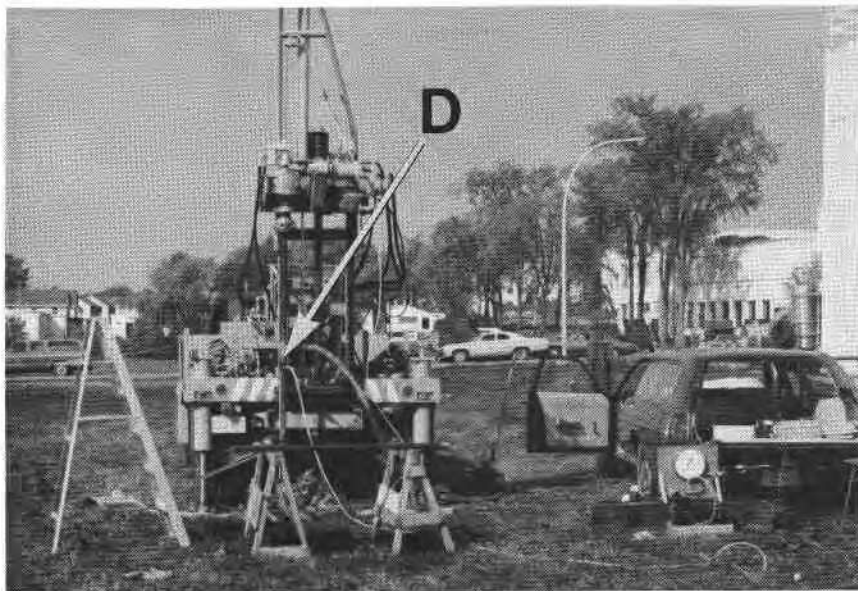
FIG. 5. Probe mounted on the drill rig. D = T-connection for the drainage hose.
