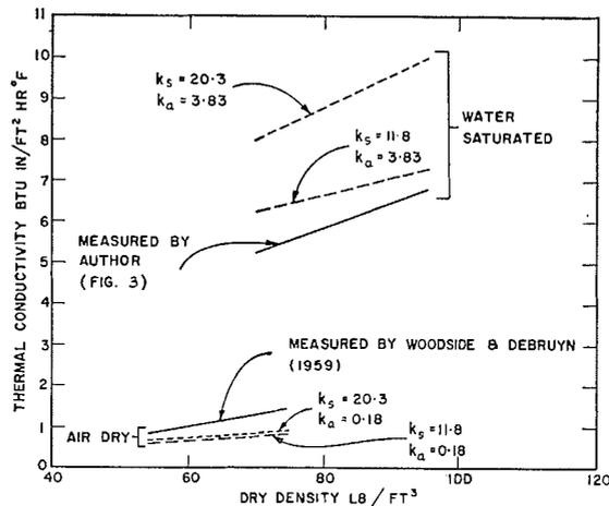
Fig. 5. Measured and calculated thermal conductivity values for air-dry and saturated Leda clay
