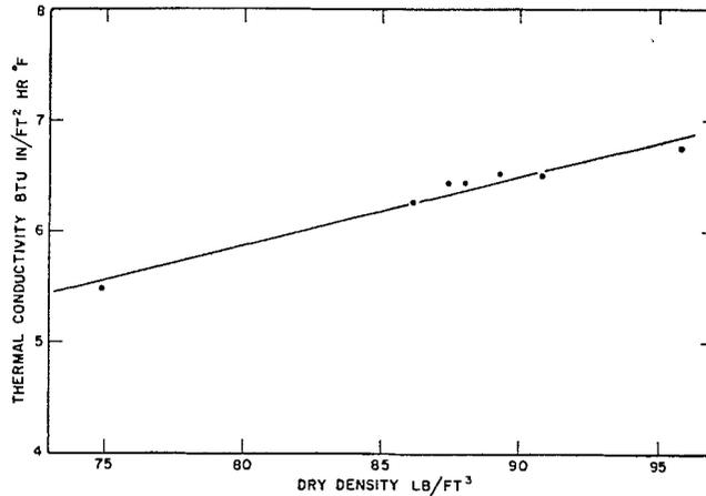
Fig. 3. Measured thermal conductivity versus dry density for saturated Leda clay
