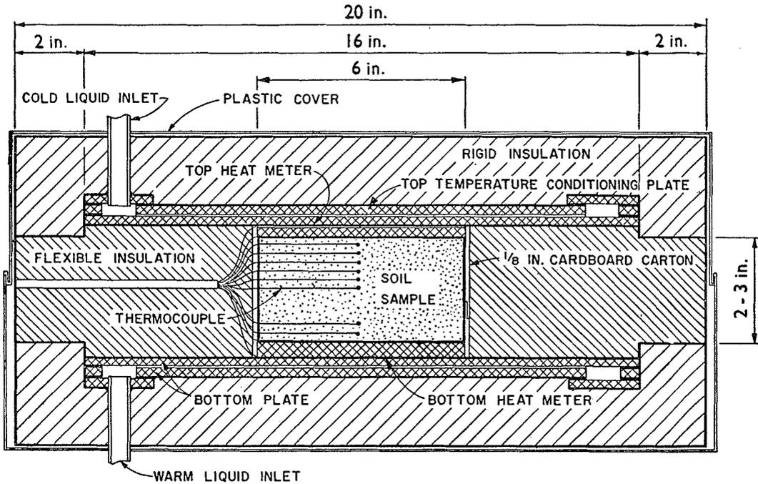
Fig. 1. Frost cell modified to measure thermal conductivity of soil (Penner 1960)
