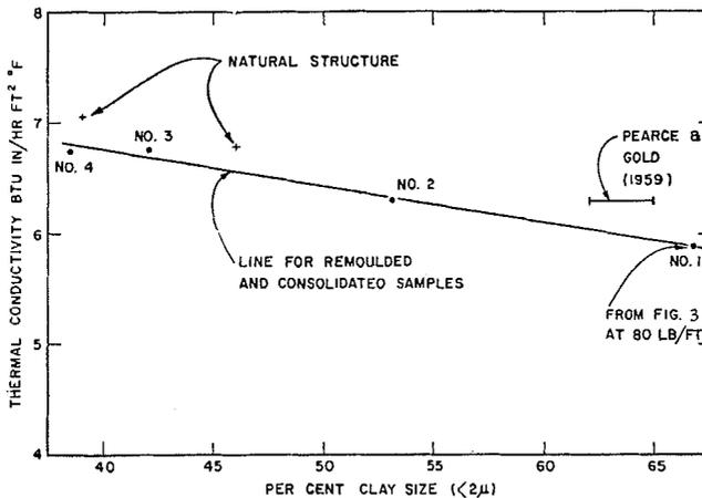
Fig. 4. Thermal conductivity versus per cent clay size (<2 microns) for saturated Leda clay at 80 lb/ft.<sup>3</sup>
