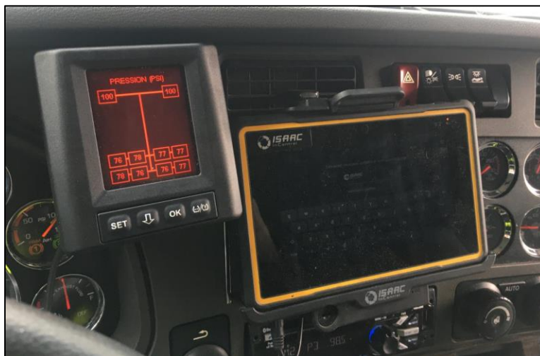
Figure 4: Continental in-cab display unit and Isaac Instruments telematics system tablet installed in truck
