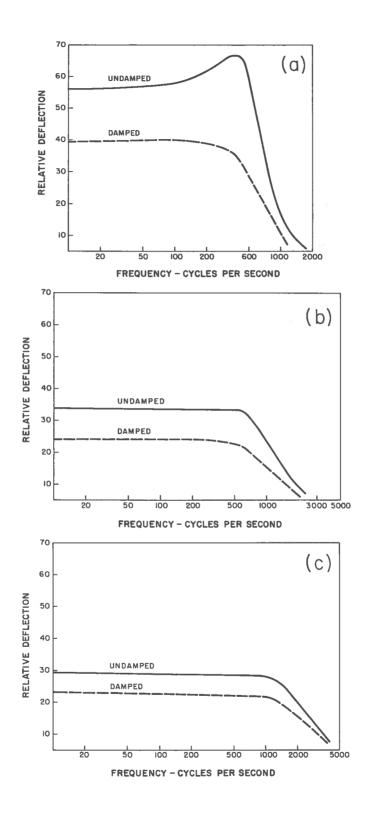
Fig. 1 Frequency response of typical galvanometers in the Sanborn optical oscillograph: (a) 350 c/s galvanometer, (b) 600 c/s galvanometer, and (c) 1200 c/s galvanometer
