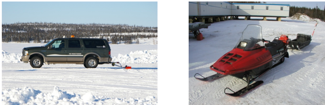
Figure 3: A ground penetrating radar (GPR) system, pulled by a light vehicle (left) or a snowmobile (right), is used to conduct high density ice, thereby closely monitoring ice thickness.
