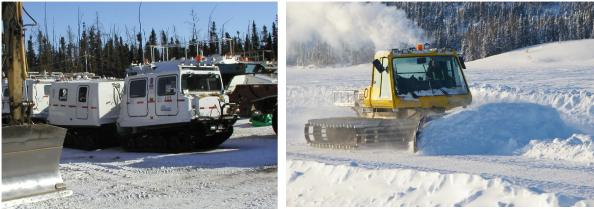
Figure 2: A Hagglund (left) and a Snow Cat (right), two light vehicles used in the initial stages of road construction to clear the ice.
