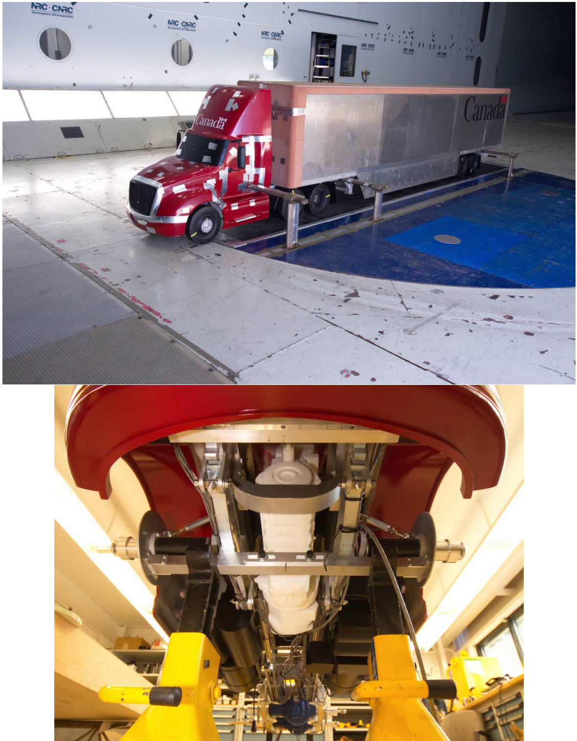
Figure 2.5: Tractor-trailer model with day-cab tractor. Top: Model overview. Bottom: Underbody details (short-sleeper-cab variant shown on jacks, without wheels).
