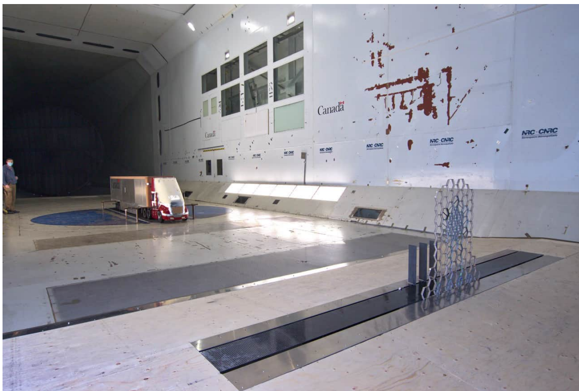
Figure 2.4: Wake-generator system, part of the NRC Road Traffic & Turbulence System, installed at the inlet of the test section (SUV-wake configuration shown).
