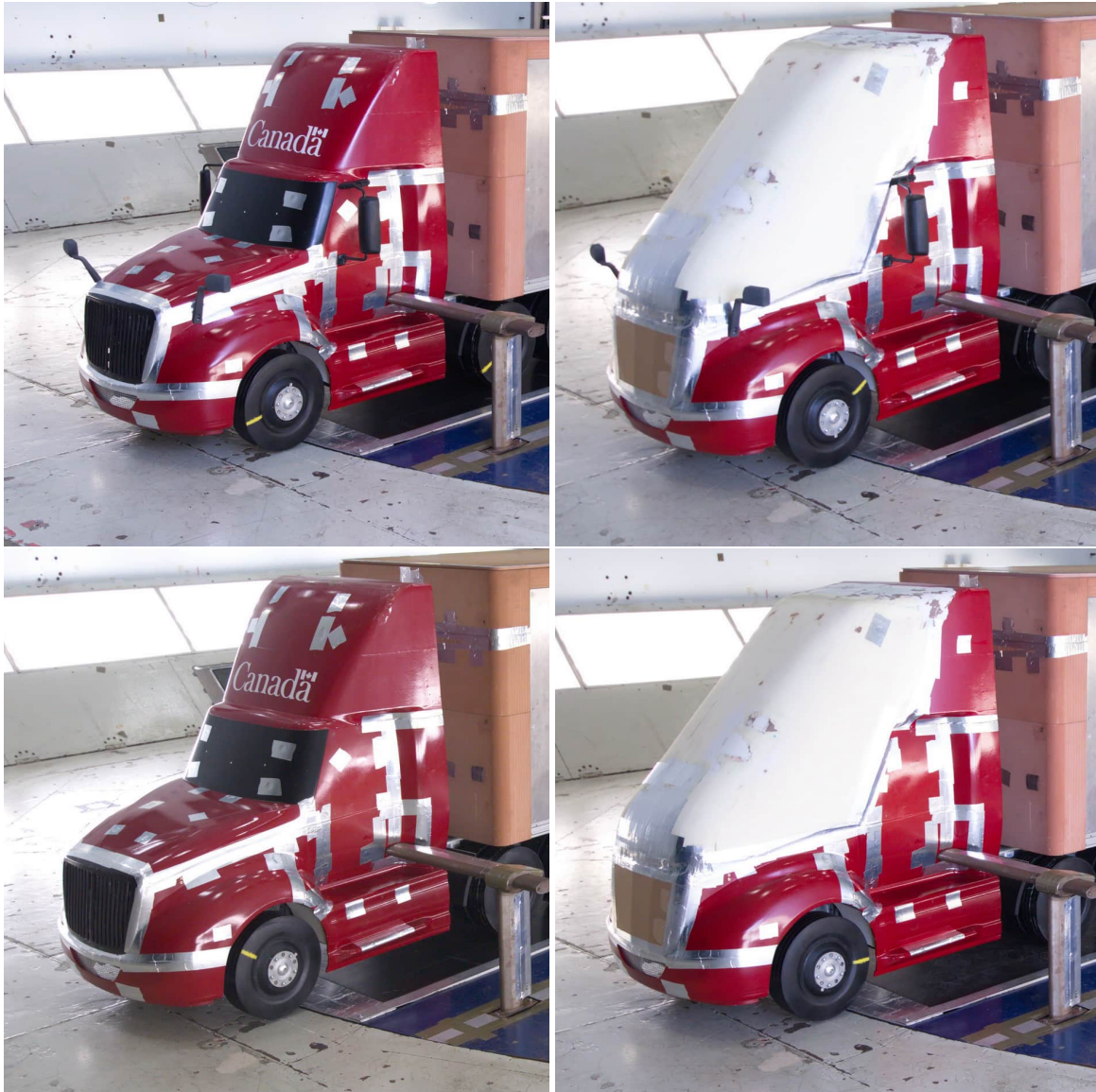
Figure 2.11: Main-mirror and fender-mirror model mounted to the day-cab (left) and zero-emission-cab (right) tractor models. Top row - both sets of mirror models installed. Bottom row - no mirror models installed.
