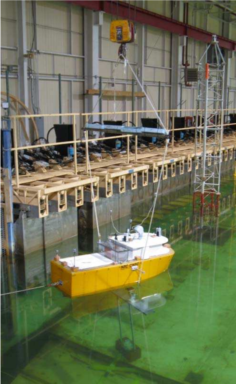
FIGURE 10: Model Launching Arrangement
