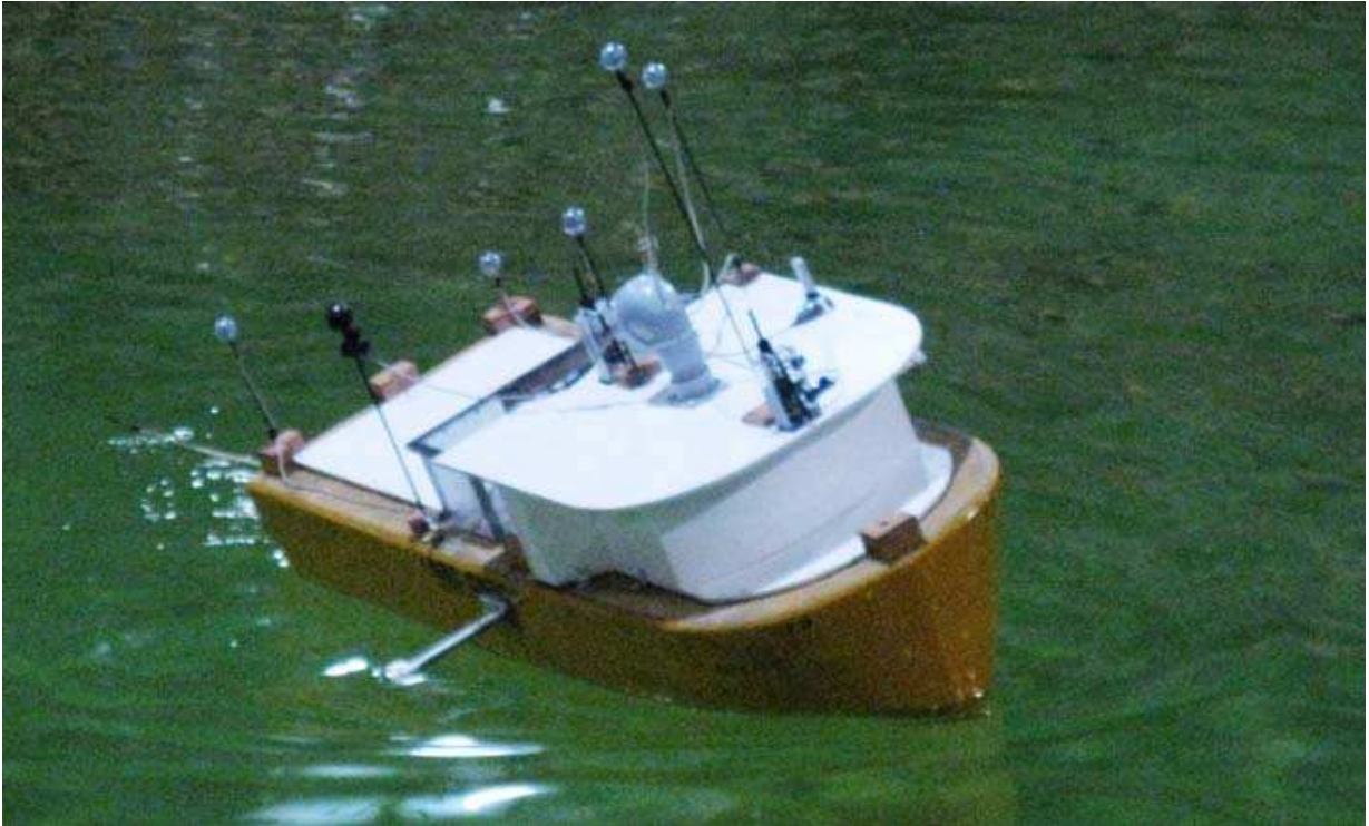
FIGURE 15: Model IOT761 During Testing – case where the period of the wave matches the natural roll period of model.
