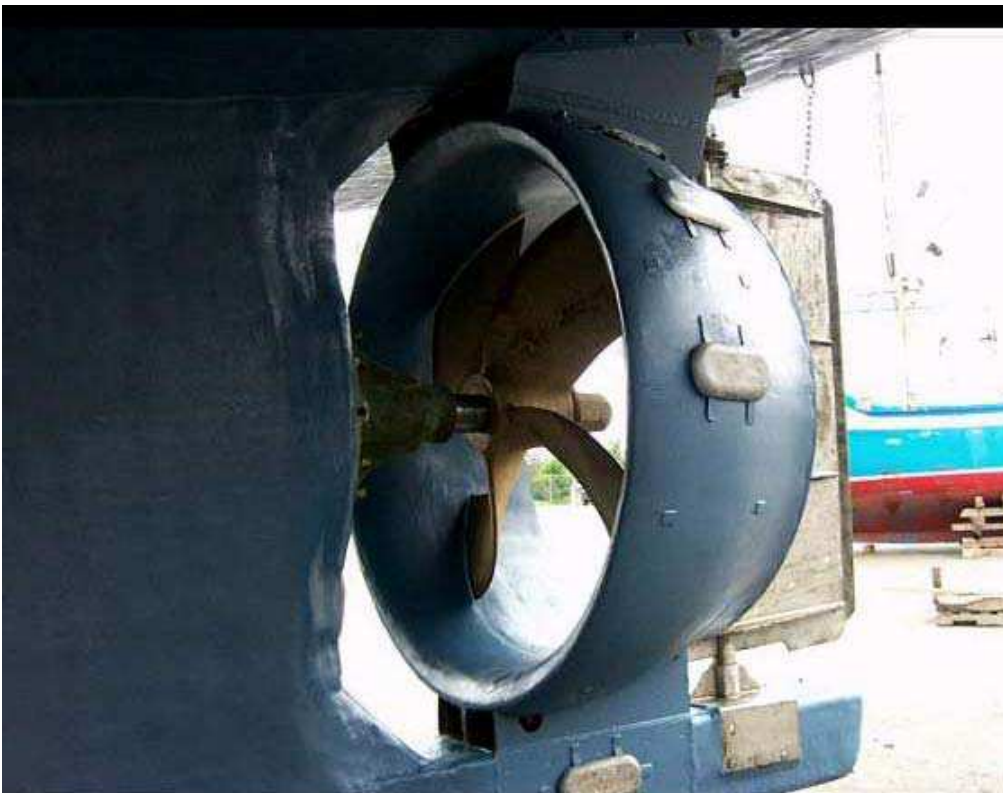
FIGURE 5: CCGA Roberts Sisters II - Propeller/Rudder Arrangement
