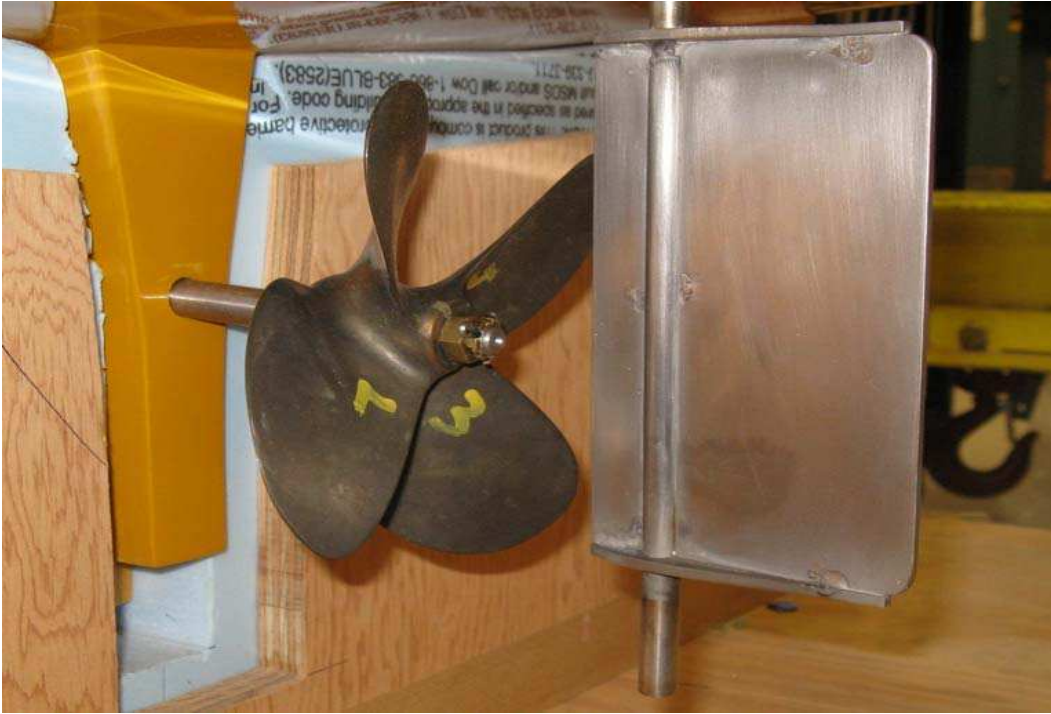
FIGURE 4: Model IOT761 Propeller/Rudder Arrangement
