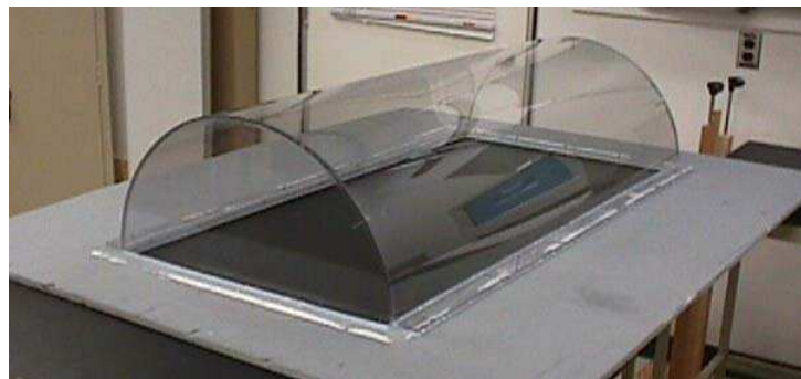
Figure 11 Barrel vault skylight as made in the laboratory.
