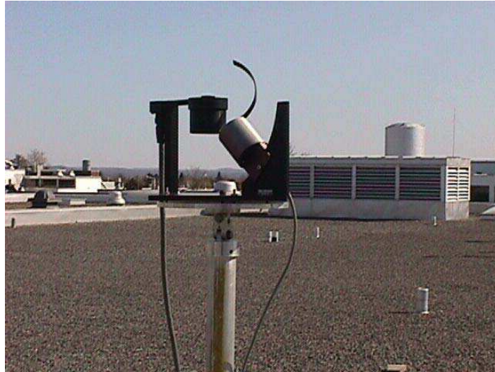
Figure 4 Solar radiation and illuminance weather station
