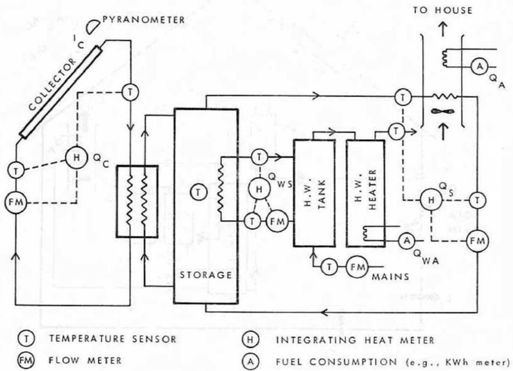
FIGURE 2 TYPICAL MONITORING EQUIPMENT LAYOUT
