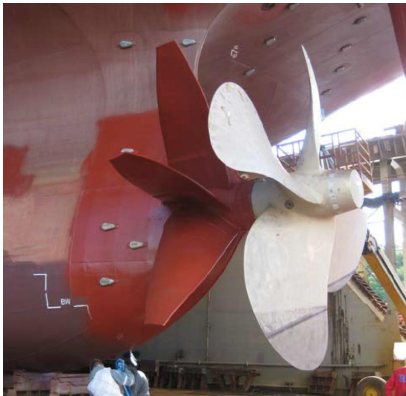
Fig.2: Pre-Swirl Stator (PSS) installed in the dry dock
