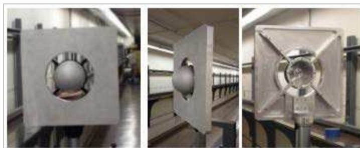
Fig. 4. Third prototype of the plate-sphere target with a 200 mm diameter integration sphere centrally mounted on a square plate with side dimensions of 609.6 mm (24 in.).
