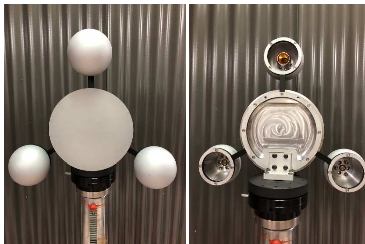
Fig. 6. Different views of the Bal-tec plate-sphere artifact presented at the annual meeting of the ASPE in 2017.
