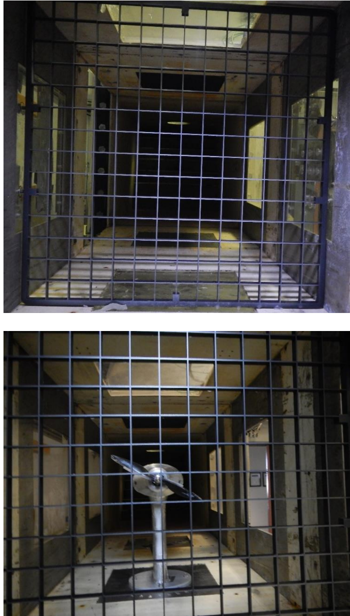
Figure 8 Grid ice collection without (upper image) and with (lower image) propeller
