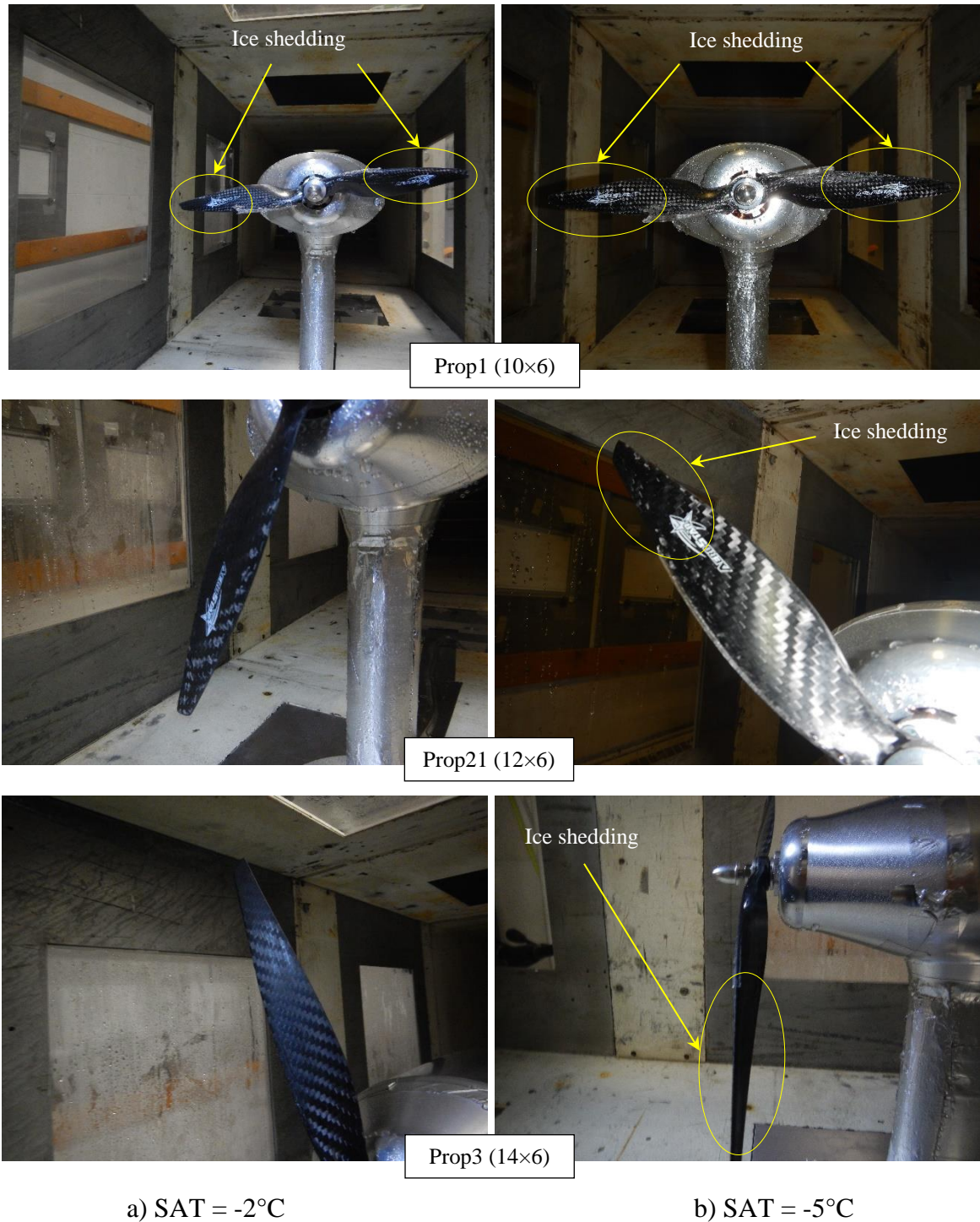
Figure 23 SAT effect on ice accretion of the three CF propellers, RPM = 8000, MVD = 20 \mu\text{m} , LWC = 0.5 \text{g}/\text{m}^3
