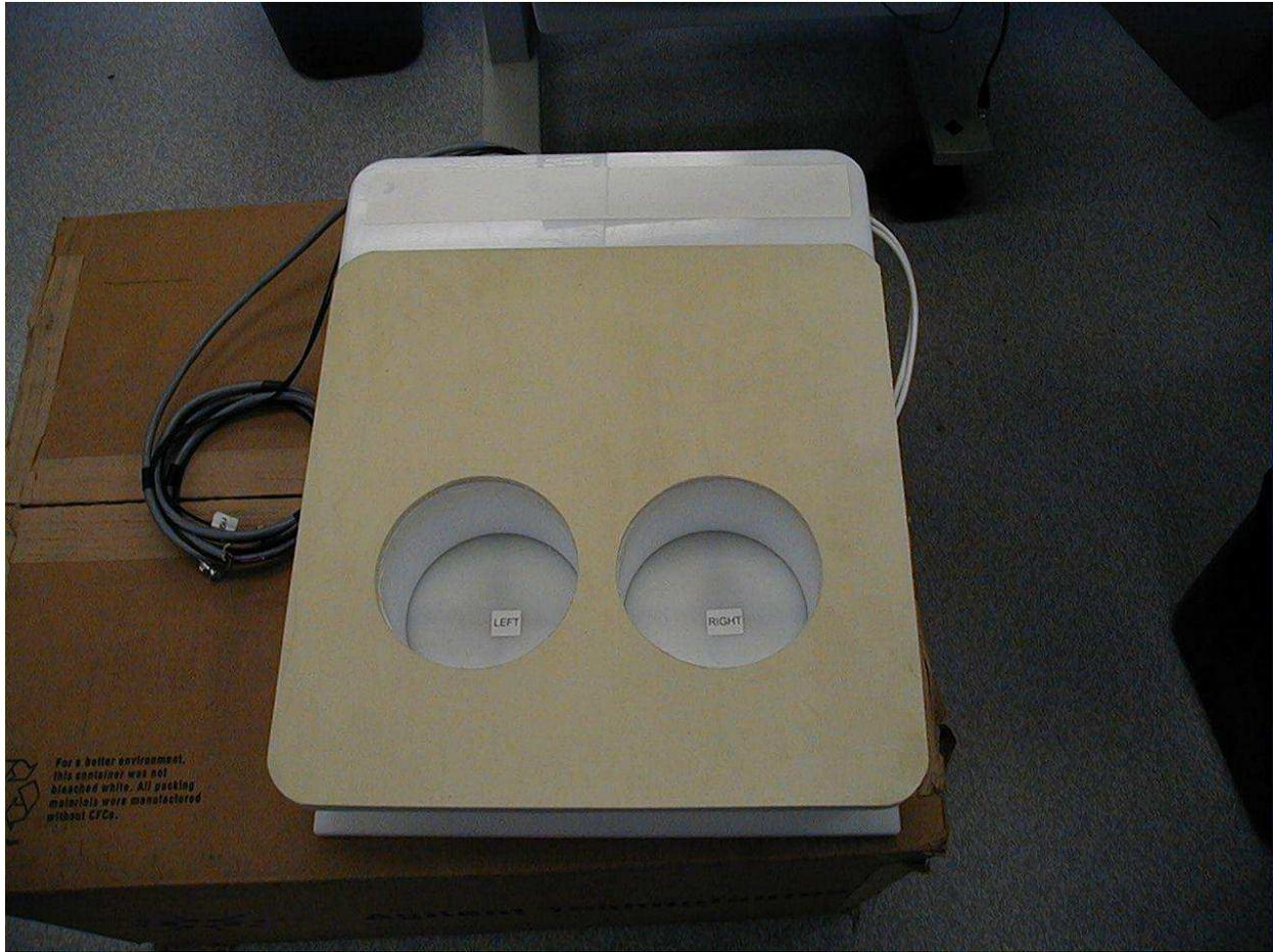
Fig.2. Picture of the breast coil.
