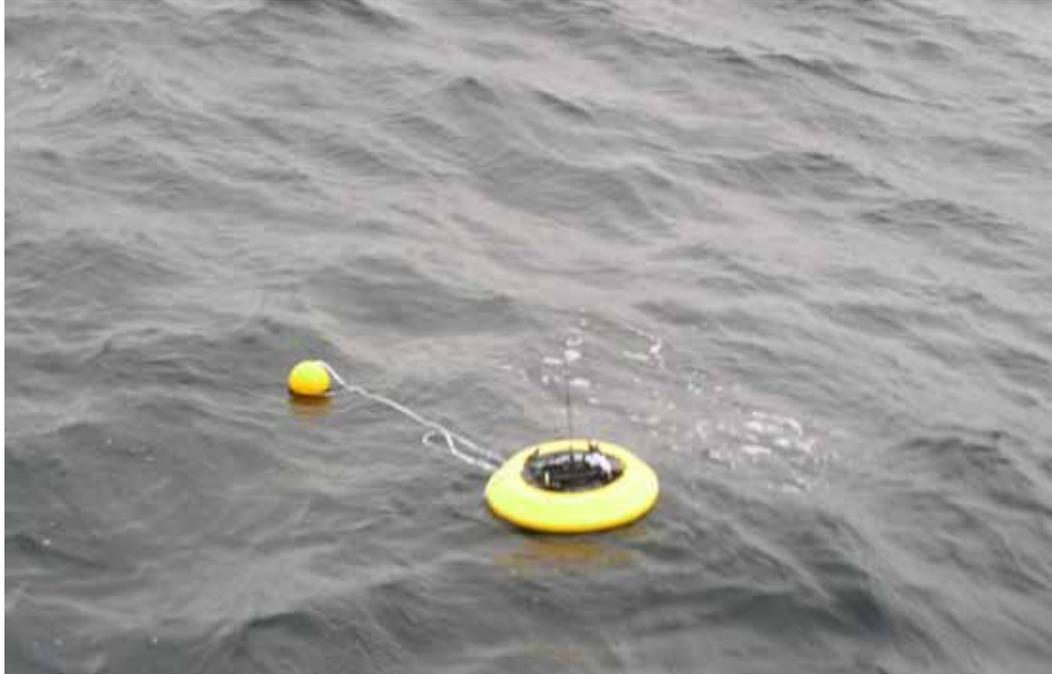
**Figure 8: Neptune Directional Wave Buoy**
