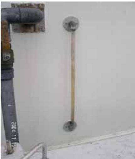
Figure 25: Anti-Roll Tank Level Indicator
