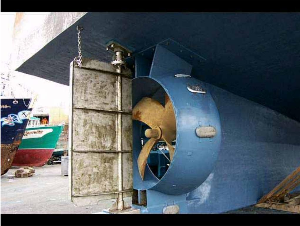
Figure 2: CCGA Roberts Sisters II – Propeller, Nozzle & Rudder Arrangement
