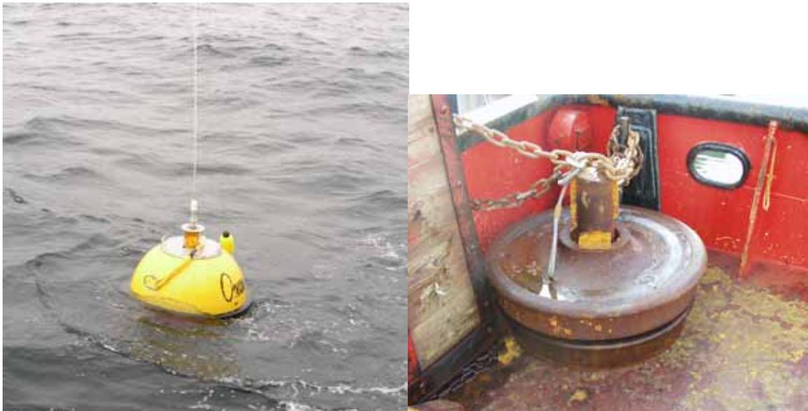
**Figure 9: Datawell Directional Wave Buoy and Anchor**
