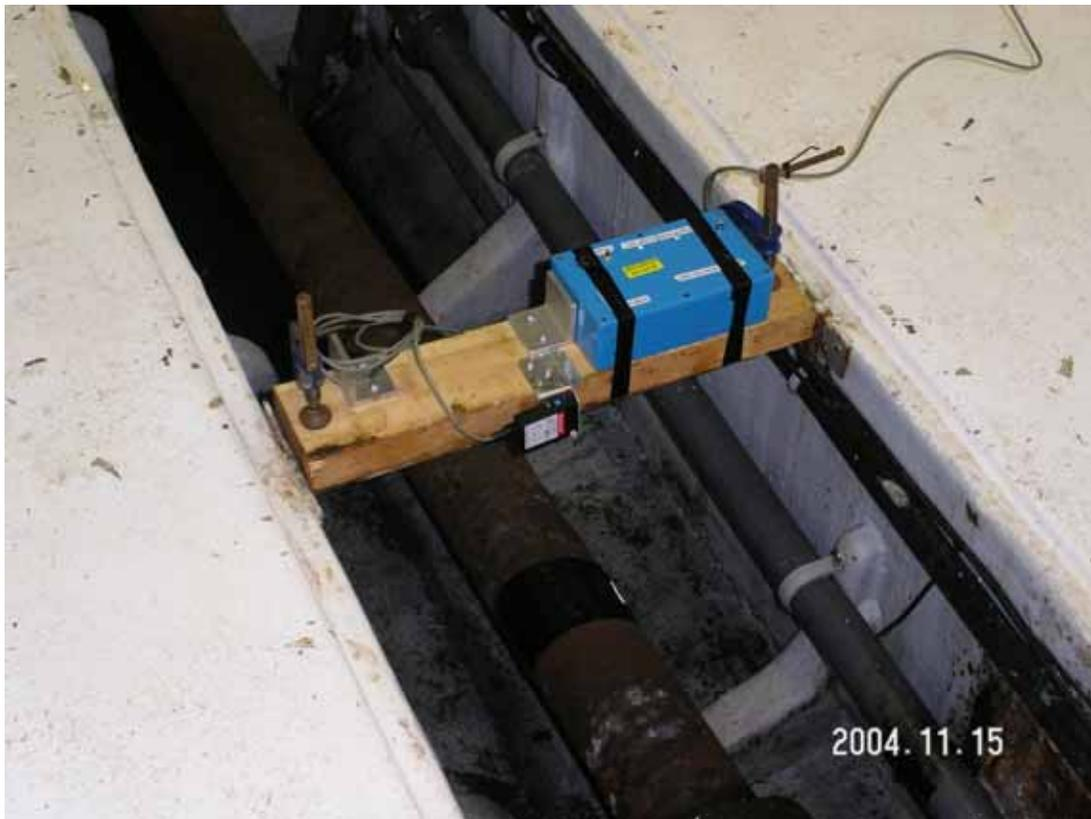
**Figure 10: Shaft RPM Measurement**
