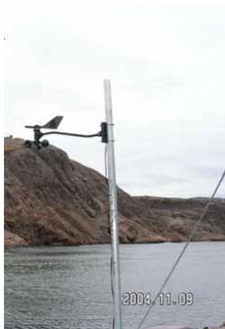
**Figure 11: Directional Anemometer**
