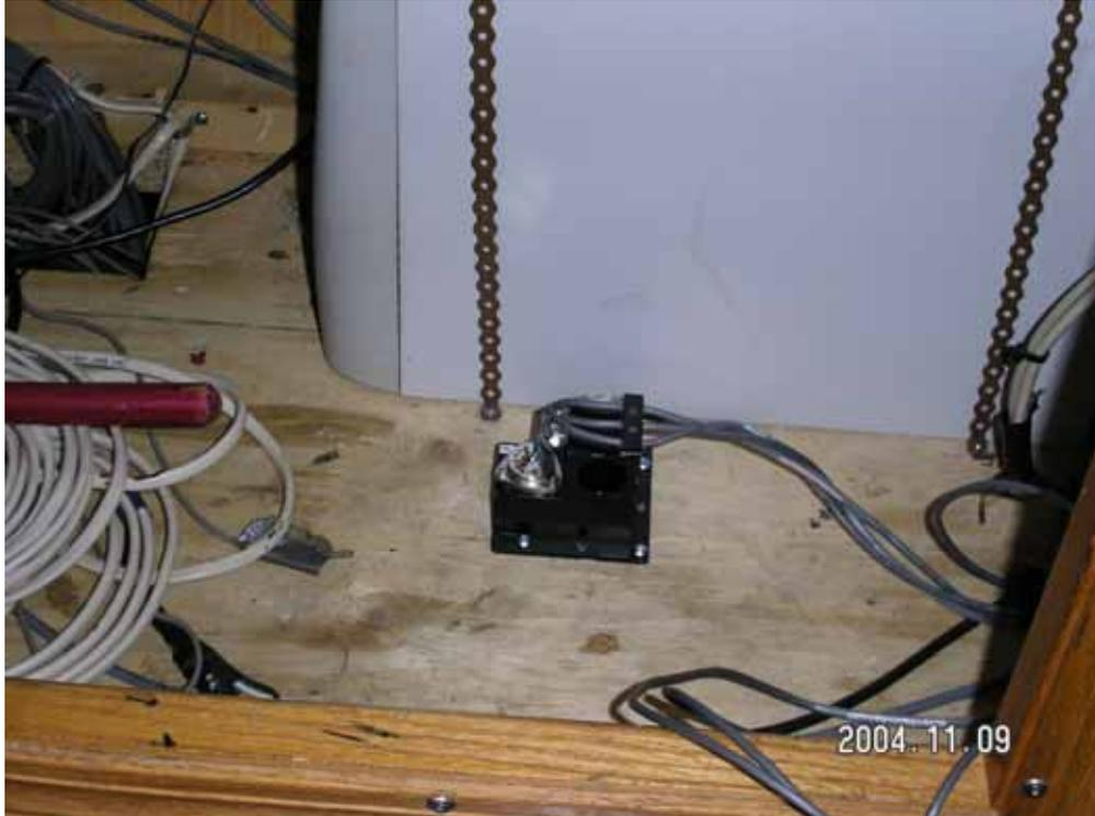
**Figure 6: Orthogonal Linear Accelerometers in Bridge Console**
