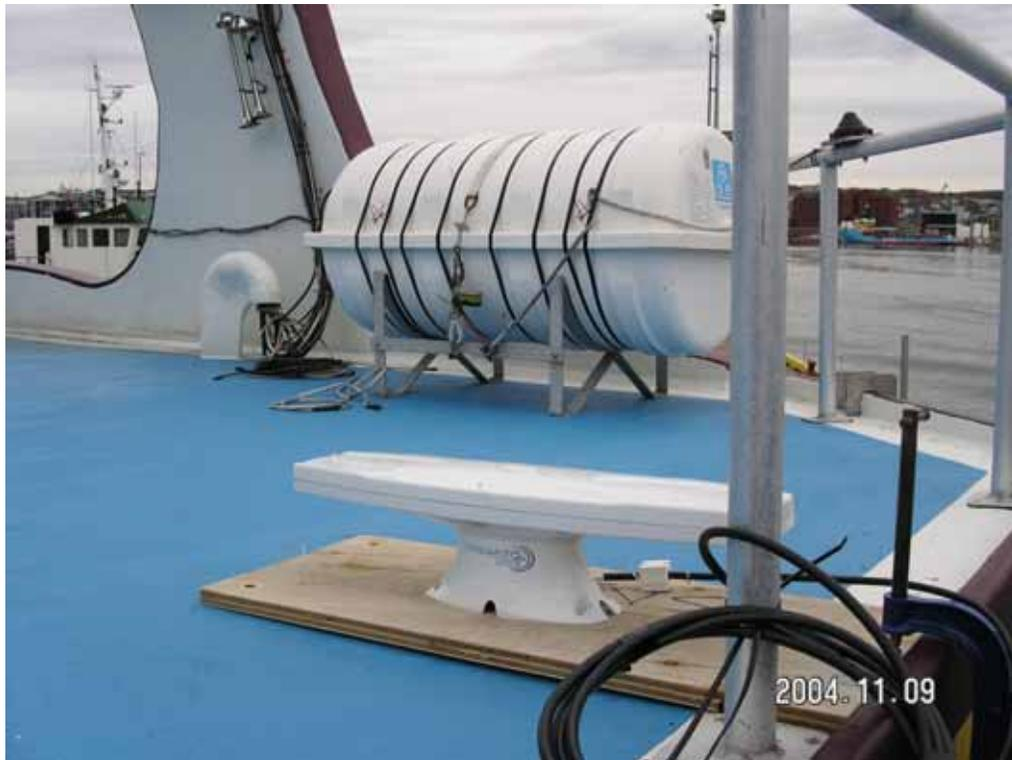
**Figure 7: DGPS Antenna on Bridge Top**
