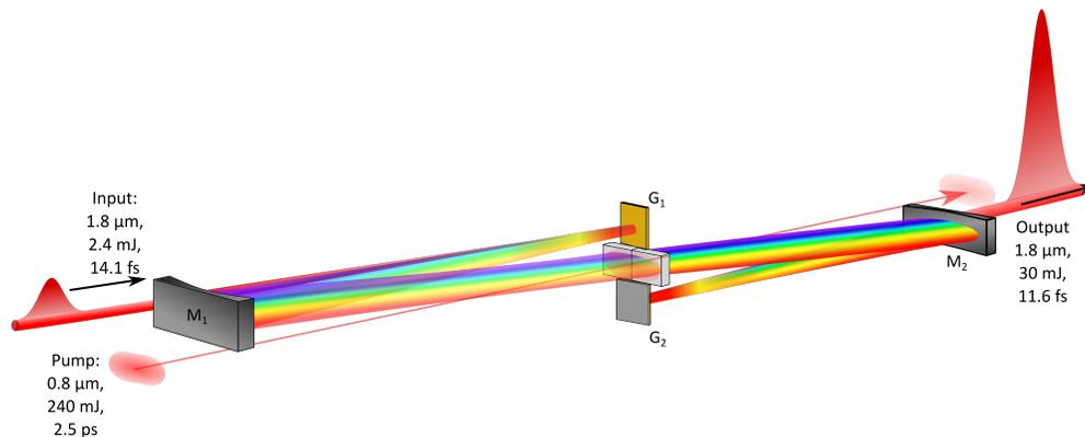
Fig. 1. A 14.1 fs, 2.4 mJ, 1.8  $\mu\text{m}$  source is injected into a 4f setup, composed of two gratings G1 and G2, and two cylindrical mirrors M1 and M2. Two BBO crystals (22x15x6 mm each) are installed in the Fourier Plane, enabling amplification up to 30 mJ with an output pulse duration of 11.6 fs, using an 800 nm, 240 mJ, 2.5 ps pump source.
