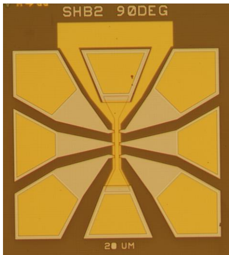
Figure 1S. A microphotograph of the second gated Hall bar sample, width of the HB channel 20 \mu\text{m} , and the distance between potential contacts 60 \mu\text{m} .
