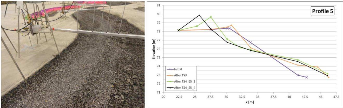
Figure 6. Typical reshaping and cross-shore profile evolution at the centre of the beach cells.
