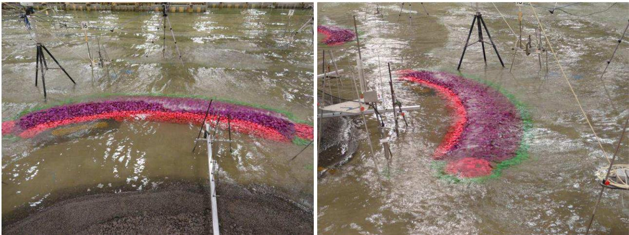
Figure 7. Overtopping of the South Island during severe conditions.
