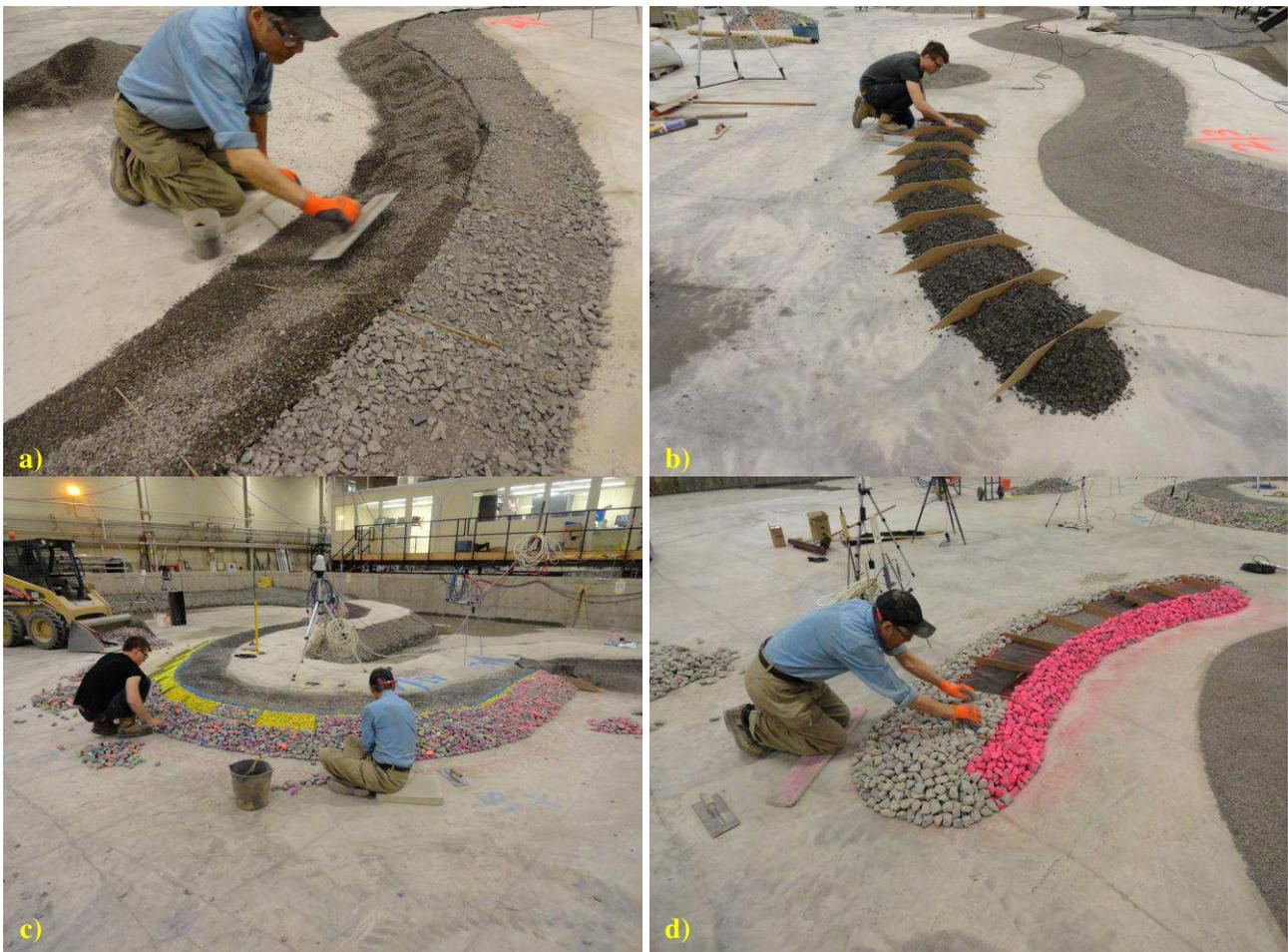
**Figure 3. Construction of coastal structures.**
