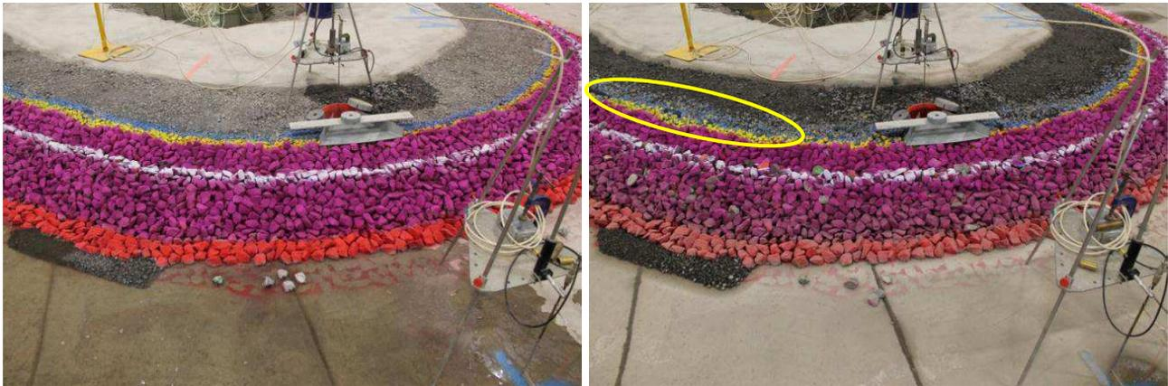
**Figure 8. Initial and final condition of the revetment headland.**
