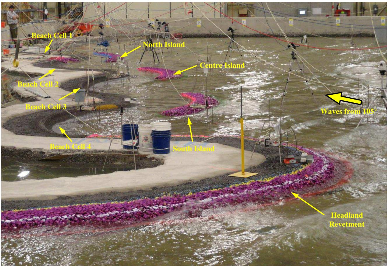
Figure 5. Testing of the Lakeview Waterfront Connection project in the NRC Large Area Basin.
