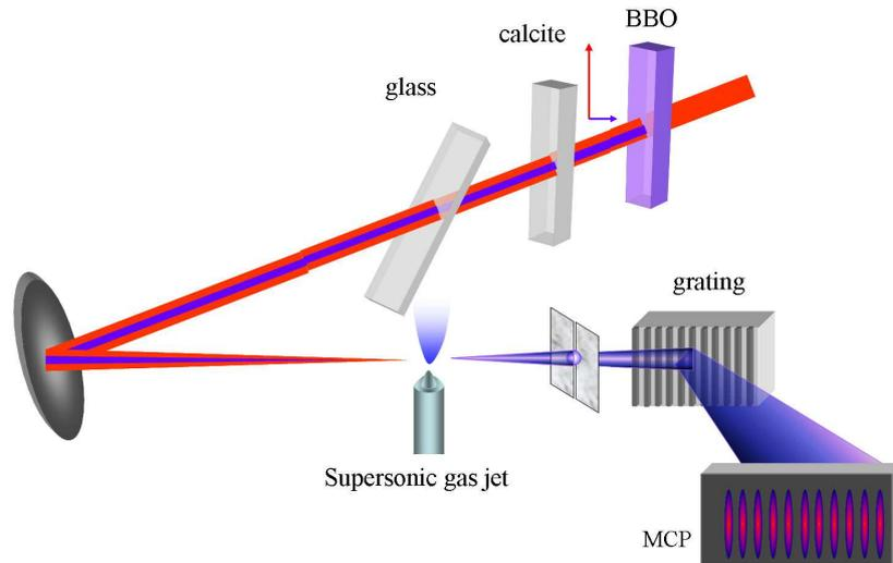
**Figure 2.** Schematic illustration of the experimental setup.
