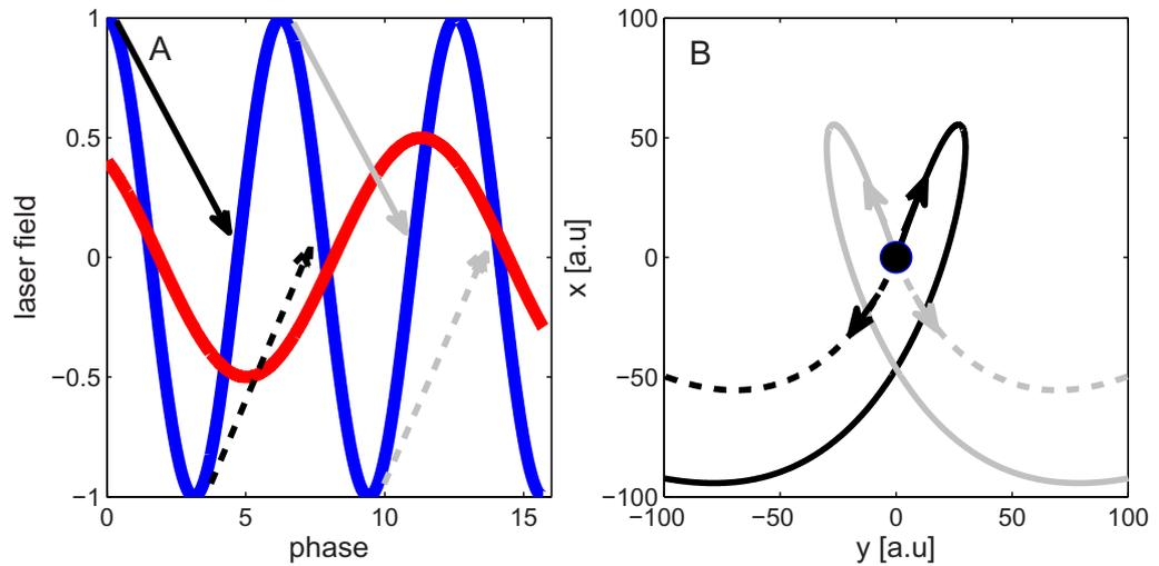
**Figure 6.** Electron trajectories in the weak fundamental–strong second-harmonic scheme. (A)  $x$ -polarized red field on a 20% intensity level of a  $y$ -polarized blue field. The four arrows represent different electron trajectories, which are plotted in panel (B). The dashed trajectories drift away from the ion, whereas the solid trajectories have large probabilities of recolliding.
