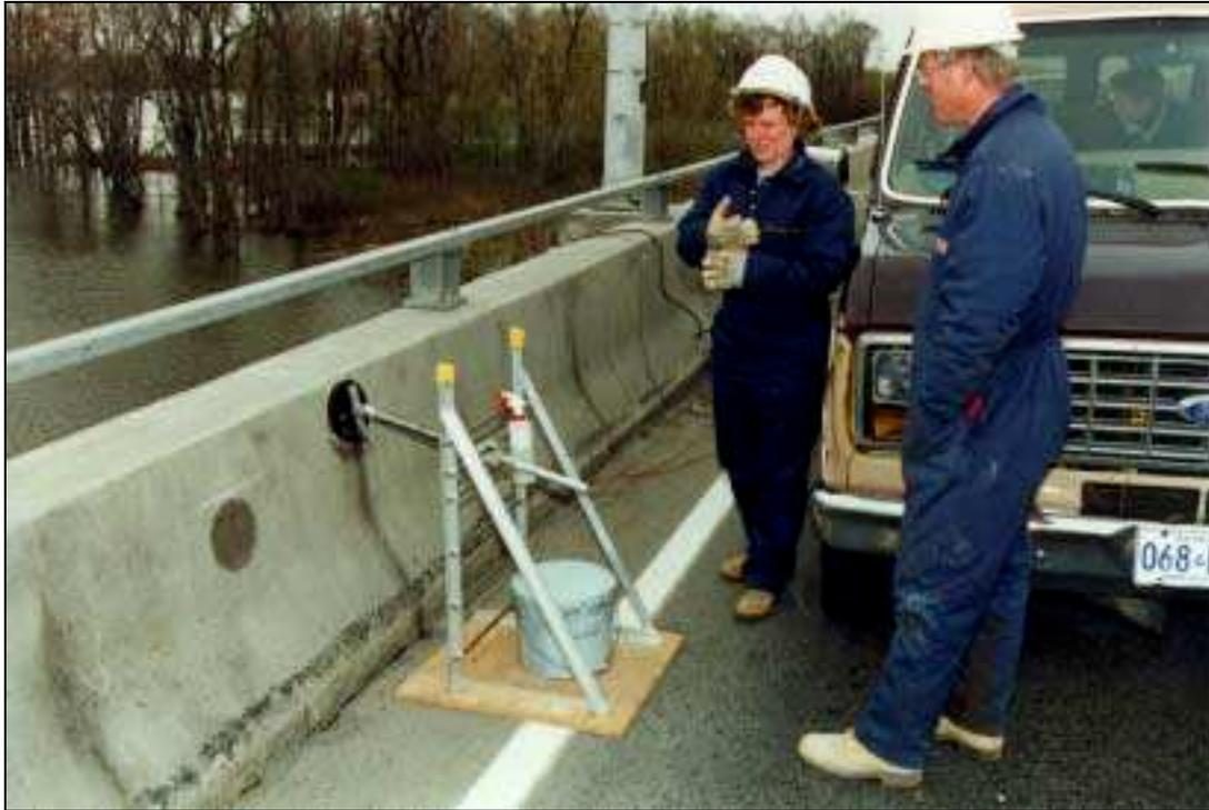
**Figure 6: Annual corrosion survey of the parapet front face**
