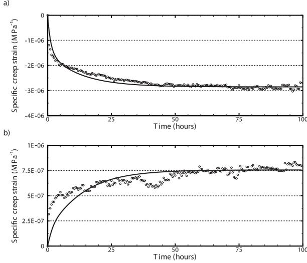
Figure 5: Parameter's identification results for the semi-graphitic carbon cathode material. a) Axial strain, b) Radial strain.  $\circ$  Experimental, — Model. From [6].
