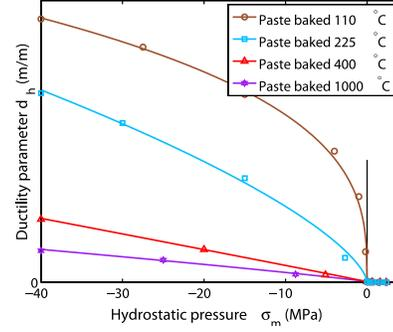
Figure 3: Evolution of the ductility curves.
