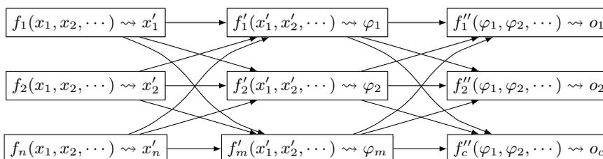
Fig. 1: Neural network representation of one specific topology containing (3) layers and  $(n + m + c)$  neurons. Each box is a neuron in the network where all activity occurs (e.g. activation, aggregation, etc). Weights are learned within the neuron by NN-GP.
