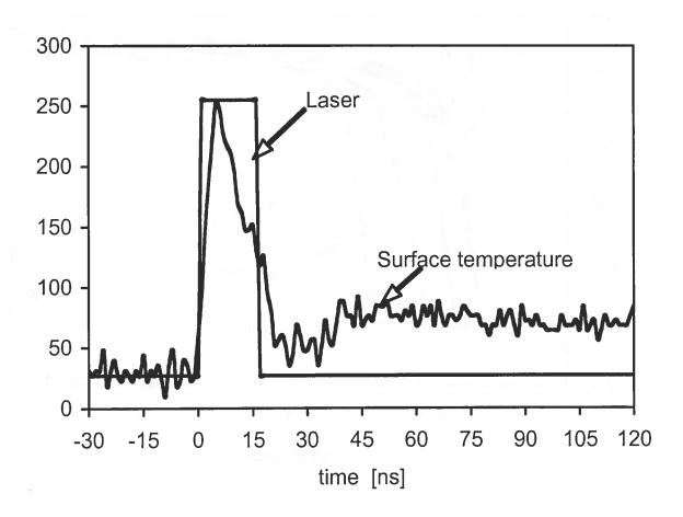
Figure 7 Thermocouple response to the application of a 46  $\mu$ J, 15 ns laser pulse applied directly to the thermocouple junction.
