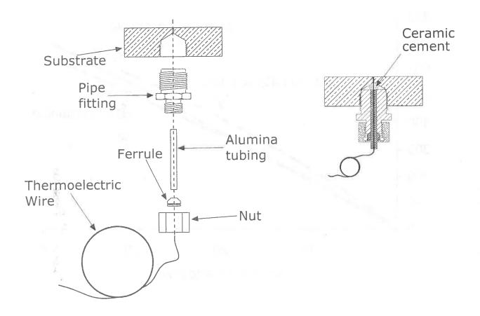
Figure 3 Thermocouple assembly
