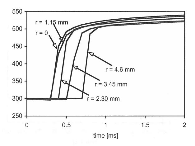
Figure 8 Response of 5 thermocouples located in a straight line at intervals of 1.15 mm from the point of impact of a 4 mm diameter molten aluminum droplet
