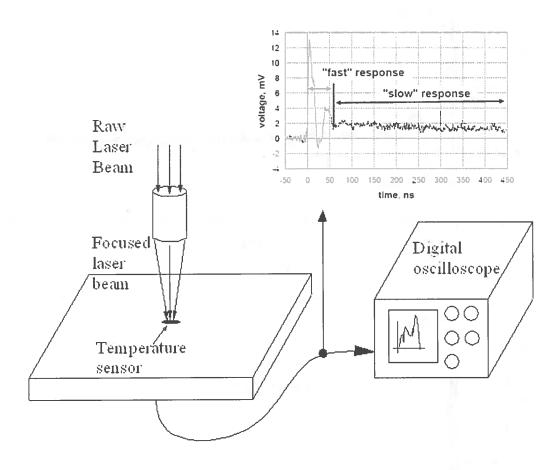
Figure 5 Schematic of experimental set-up for response time measurement.
