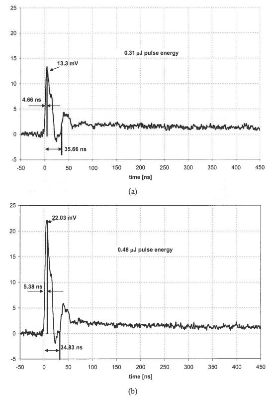
Figure 6 Typical response functions of the thermocouple with a) 0.31  $\mu$ J pulse energy and b) 0.46  $\mu$ J pulse energy
