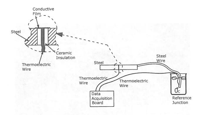
Figure 1 Schematic diagram of thin-film thermocouple.
