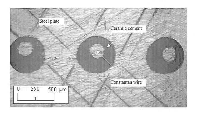
Figure 2 Top view of three temperature sensors placed 1.15 mm apart,.
