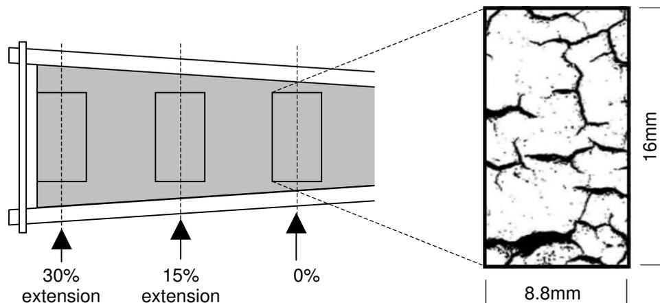
Figure 7. Measurement position of crack area of sealant
