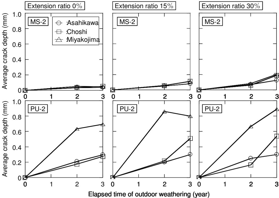
Figure 11. Relation between elapsed time and average crack depth of sealant
