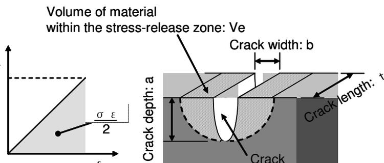
Figure 13. Schematic showing the volume of sealant within the stress-release zone
