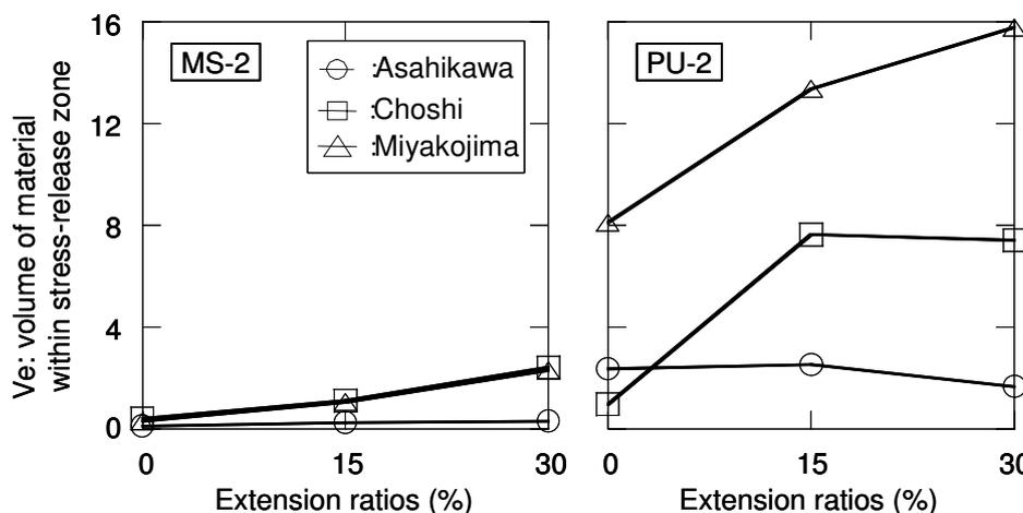
Figure 14. Result of calculation of the volume ( $V_e$ ) within the stress-release zone (Exposure period, 3-years)
