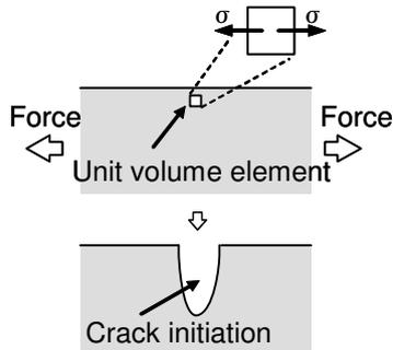
Figure 12. Strain energy of unit volume element
