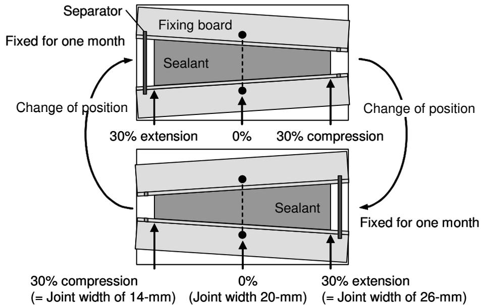
**Figure 2. Sealant specimens subjected to continuous joint movement**
