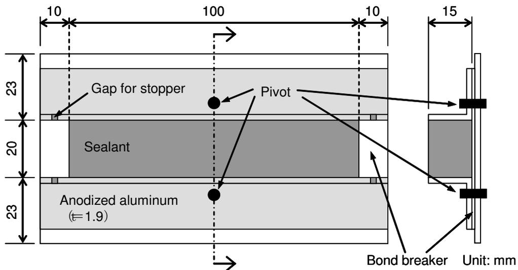
Figure 1. Variable movement test specimen
