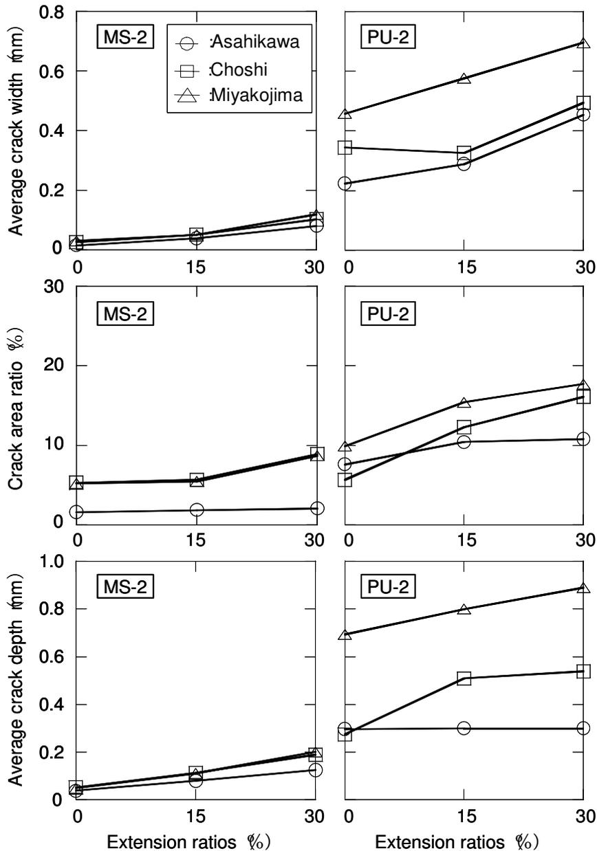
Figure 10. Results of surface condition of sealant after 3 years exposure
