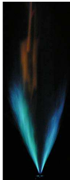
Figure 1: Rod-stabilized V-flame with a rich to lean mixture fraction gradient from left to right
