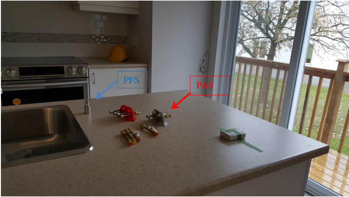
Fig. A. 7. Passive flux sampler (PFS) and passive air sampler (PAS) in the duplex research house (kitchen, 1st floor).
