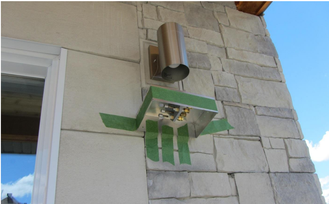
Fig. A. 8. Passive air sampler (PAS) outside of the duplex research house.
