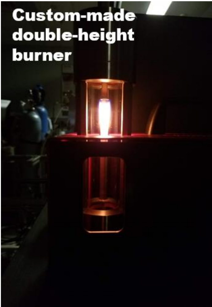
Figure S2. Photograph of the custom-made double-height burner.
