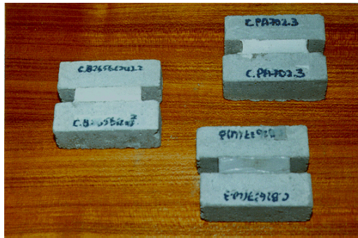
Fig. 2: H-joint configuration sealant specimens with different types of substrates i.e. glass, mortar and aluminium prepared similar to that of ASTM C719-93
