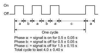
Figure 2. Temporal-Three pattern for fire evacuation alarm signal
