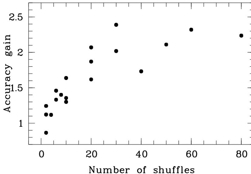
Figure 1: The DAO spectropolarimeter uses fast modulation in order to fight instrumental effects. The relative increase in positional accuracy versus the number of switch cycles is shown in this figure. With 20 or more switch cycles the accuracy improves by a factor of two or more.
