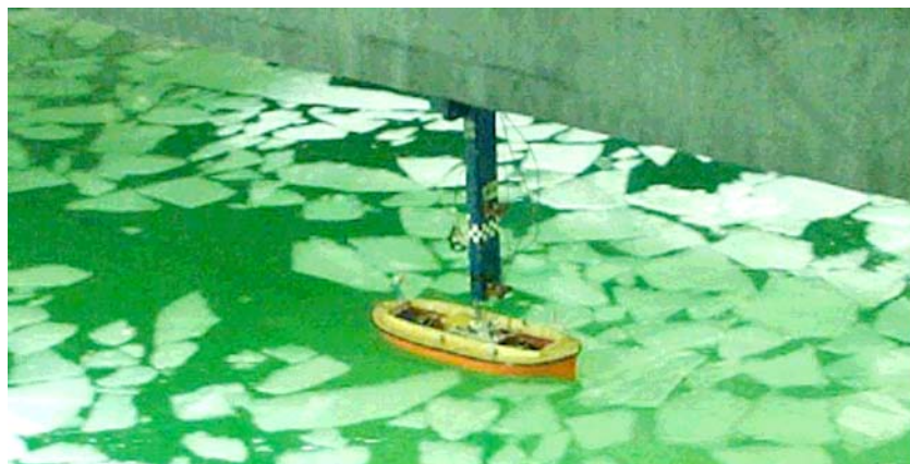
Figure 3: Conventional TEMPSC lifeboat 1:13 scale model.
