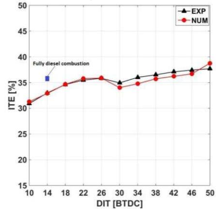
**Fig. 6:** ITE vs. diesel injection timing for natural gas/diesel dual-fuel mode at 25% engine load.
