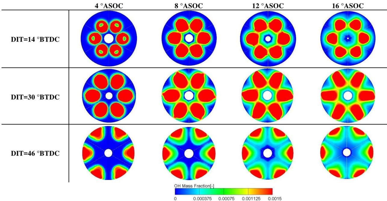
**Fig. 5:** Spatial contours of OH radical for various diesel injection timings under 25% engine load.
