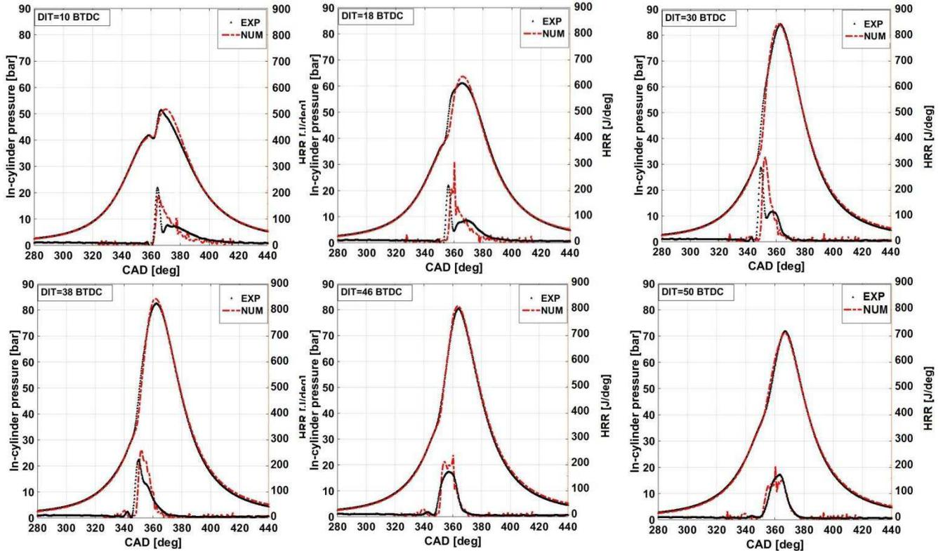
Fig. 2: Experimental and numerical in-cylinder pressure and HRR at different injection timings under 25% engine load.
