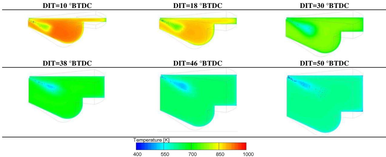
**Fig. 3:** In-cylinder temperature contours (at 5 °CA ADIT) for various diesel injection timings under 25% engine load.
