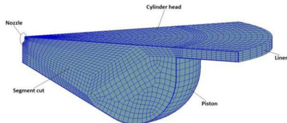
**Fig. 1:** Computational domain of the combustion chamber at the TDC.
