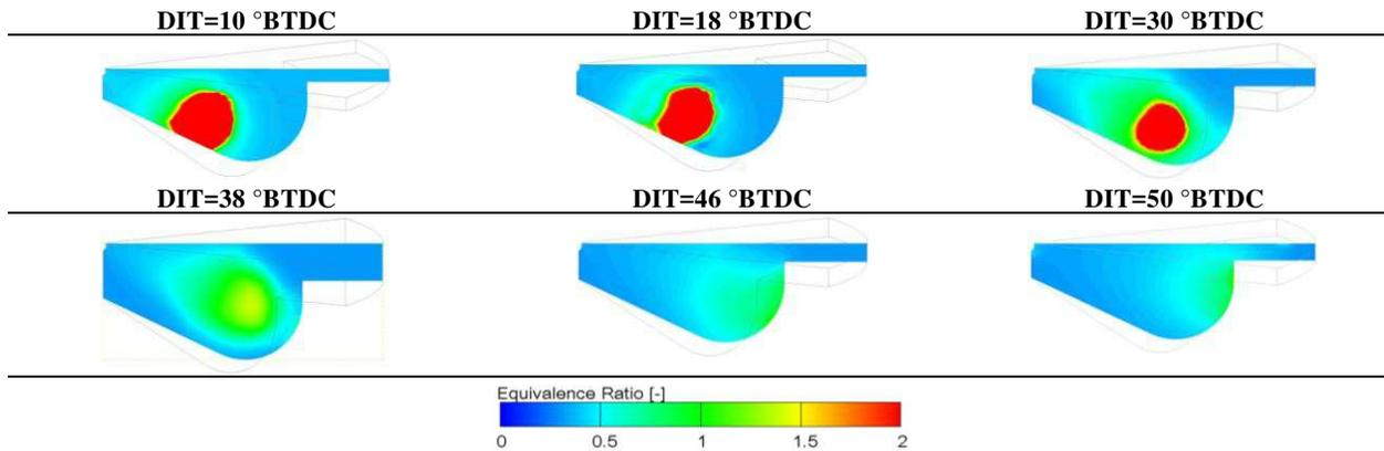
**Fig. 4:** Spatial contours of total equivalence ratio (at SOC timing) of various diesel injection timings under 25% engine load.
