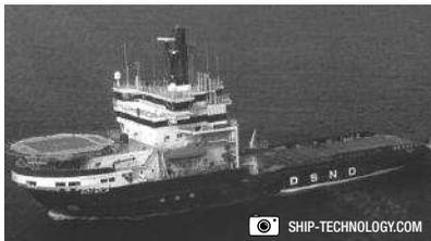
Fig. 25. The Finnish icebreaker *Botnica*, the first to use Azipod propulsion in 1998.
