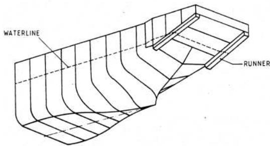
Fig. 22. The Thyssen-Waas icebreaking concept (above) and the Max Waldeck with a Waas bow (below).
