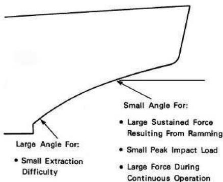
Fig. 12. The "White" bow as used on the *Manhattan* (White, 1969, 1970).
