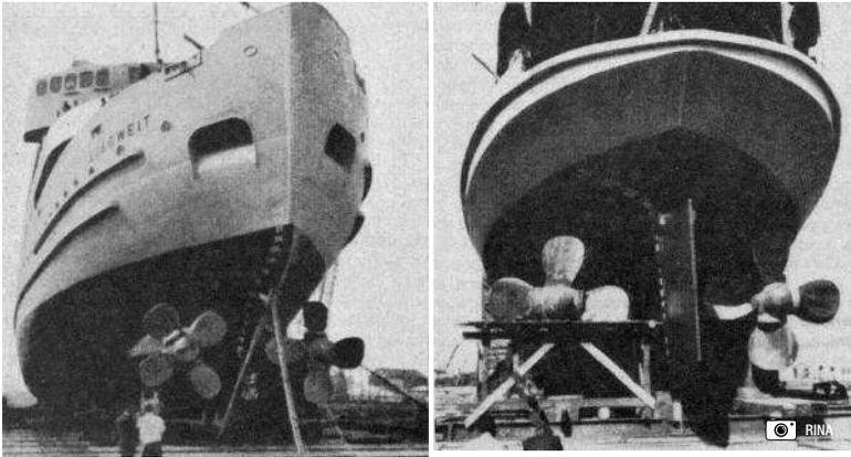
Fig. 7. The bow and stern of the *Abegweit* showing the two bow and stern propellers (Jansson 1956).
