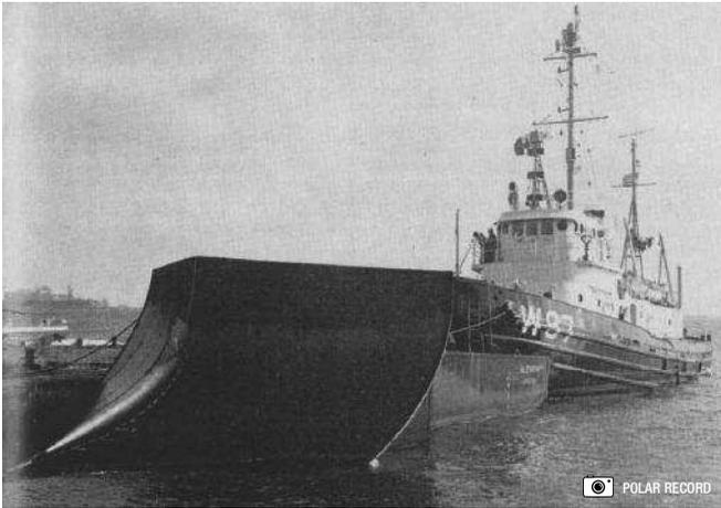
Fig. 11. Tug fitted with Alexbow icebreaking device.
