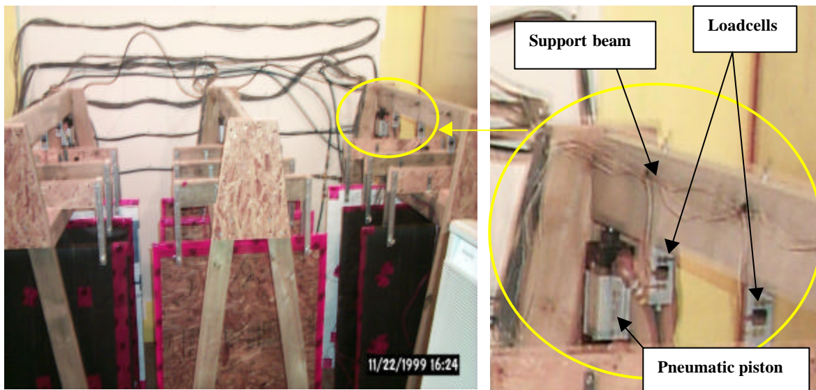
Figure 8 — Automated-weighing system for mid-scale specimens showing load cell support beams, load cells, pneumatic pistons and specimen holders.
