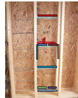
Figure 25– W6: Response of moisture detection strip to the presence of moisture in the wall
