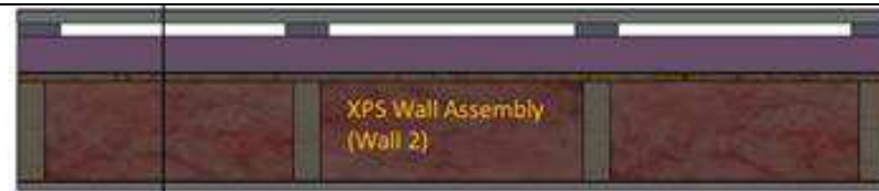
Figure 2. Schematic of three 38 mm x 140 mm (2 x 6 in.) wood-frame wall (residential) test specimens installed side-by-side in FEWF
