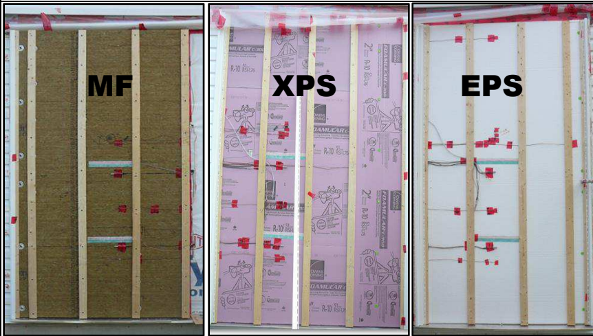
Figure 8. Installation of W1, W2, & W3 in FEWF showing respective insulation panels including EPS (W1), XPS (W2) and MF (W3)
