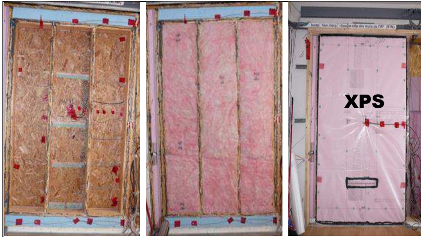
Figure 14. Wall 4 (XPS) – Interior wood frame prior to (i) & following installation GF batt insulation in stud cavities (ii), & placement of 51 mm of XPS insulation & PE vapour barrier (iii)
