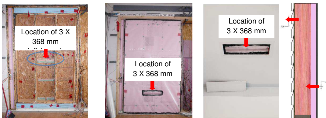
Figure 18 – Deficiencies in wall test specimens showing location & size of deficiency in W4 (XPS)
