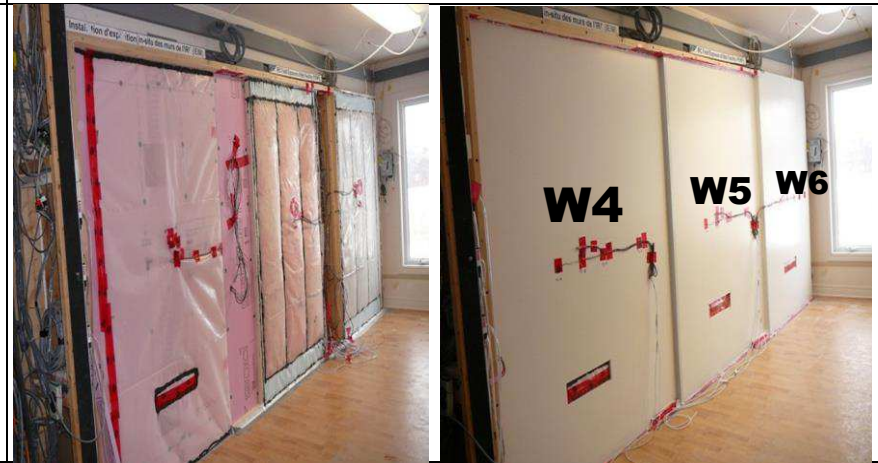
Figure 17. Interior of FEWF showing W4 (XPS), W5 (SPF), and W6 (CFI) prior to (i) & following (ii) installation of interior drywall
