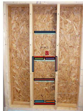
Figure 24– W5: Response of moisture detection strip to the presence of moisture in the wall
