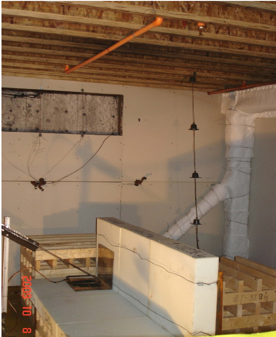
Figure 73. Sprinkler and CPVC piping relative to exposed wood I-joists and fuel (Test PF-03B)
