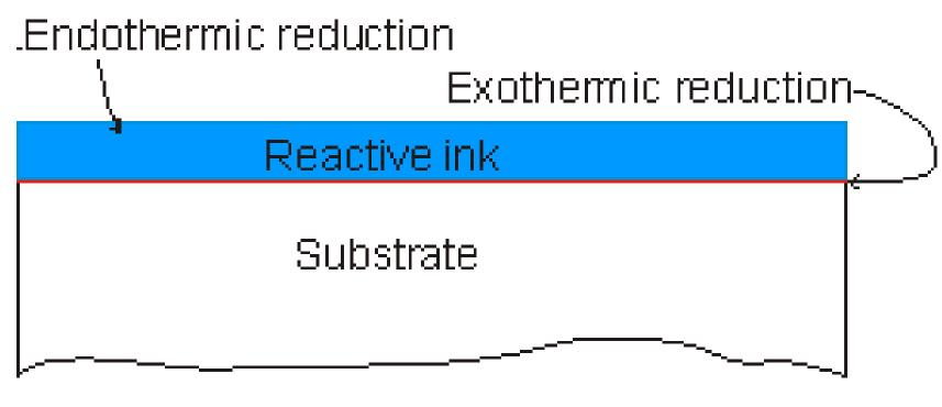
**Figure 1.** The design of a silver deposition process that doesn't need external heat
