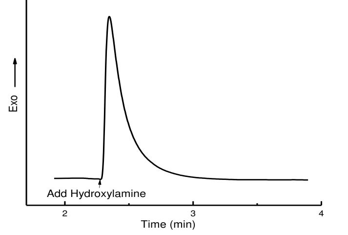
Figure 2. DSC trace of the reactive silver ink at room temperature when hydroxylamine was added.
