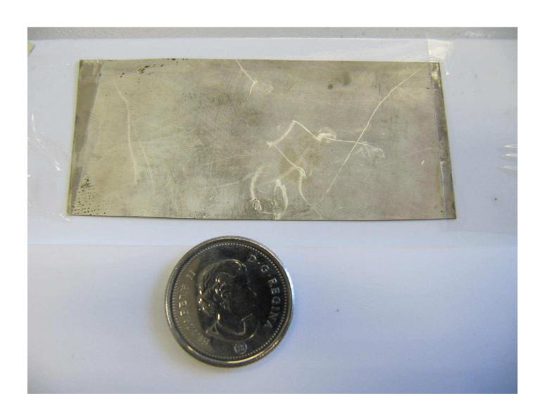
Figure 4. Silver film deposited on PET film using the reported process. PET films from Novacentrix were used.
