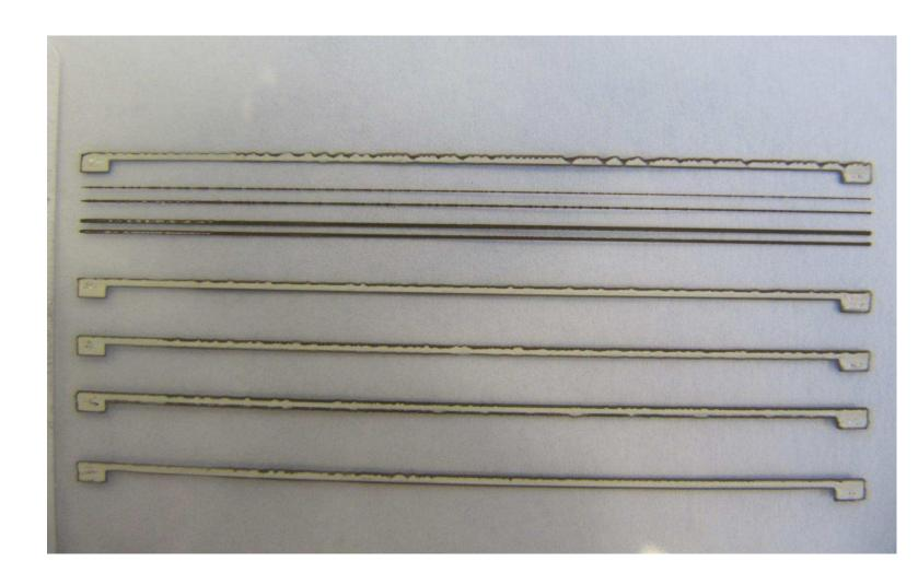
As the described silver deposition happens at room temperature, it is possible to print silver patterns on papers. Commercial photo printing papers with smooth surface and nano pores were tested suitable for the application. Figure 6 shows the silver lines printed on Canon photo paper. With the addition of a suitable surfactant, the line quality could be substantially improved.
