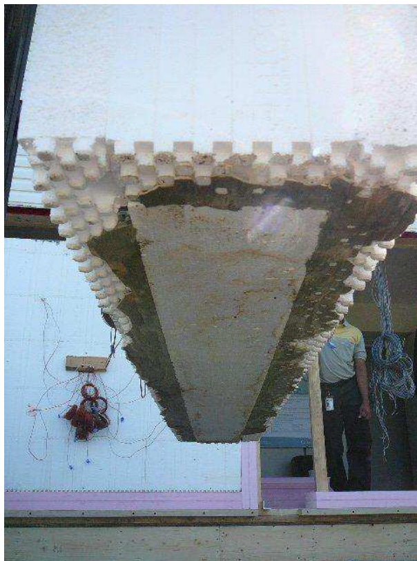
Figure A-23. View of the bottom of the second ICF wall specimen as it is being lifted into position.
