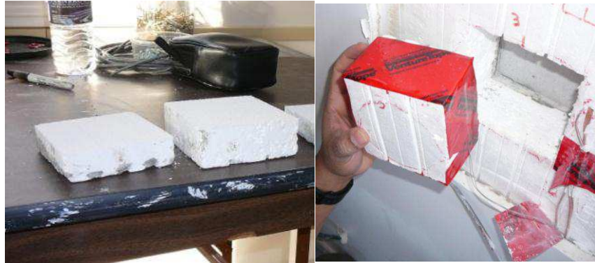
Figure 5. Heat flux transducer repositioned in the middle of the EPS
