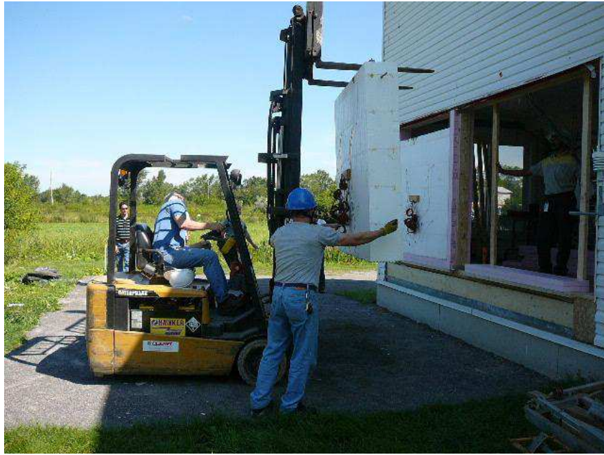
Figure A-24. Lifting the second ICF wall specimen into position.
