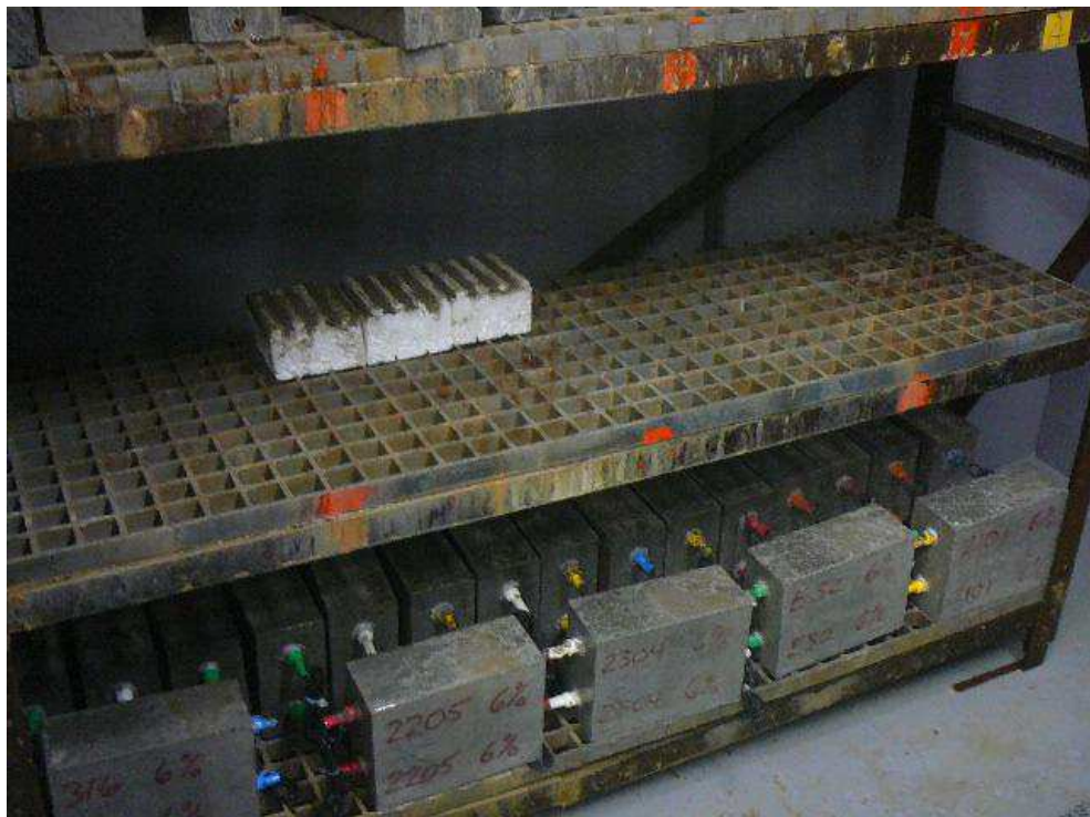
Figure A-59. Curing the concrete in controlled conditions.
