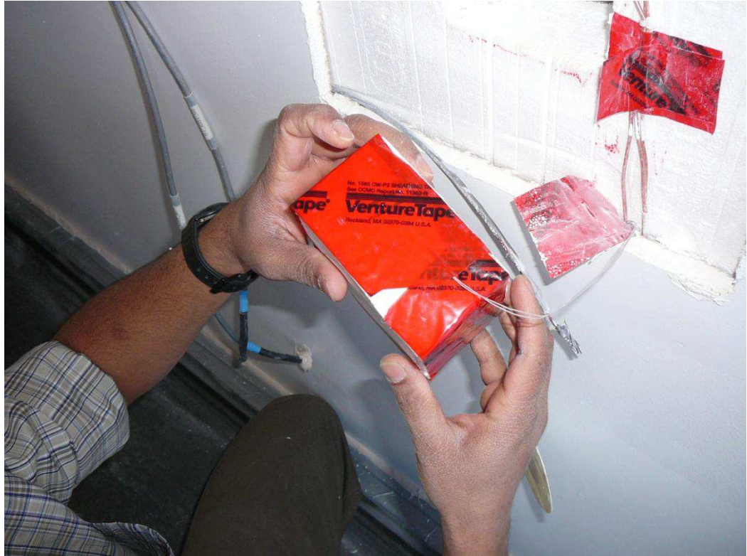
Figure A-66. Repositioning of the heat flux centre between the two sections of the foam block.
