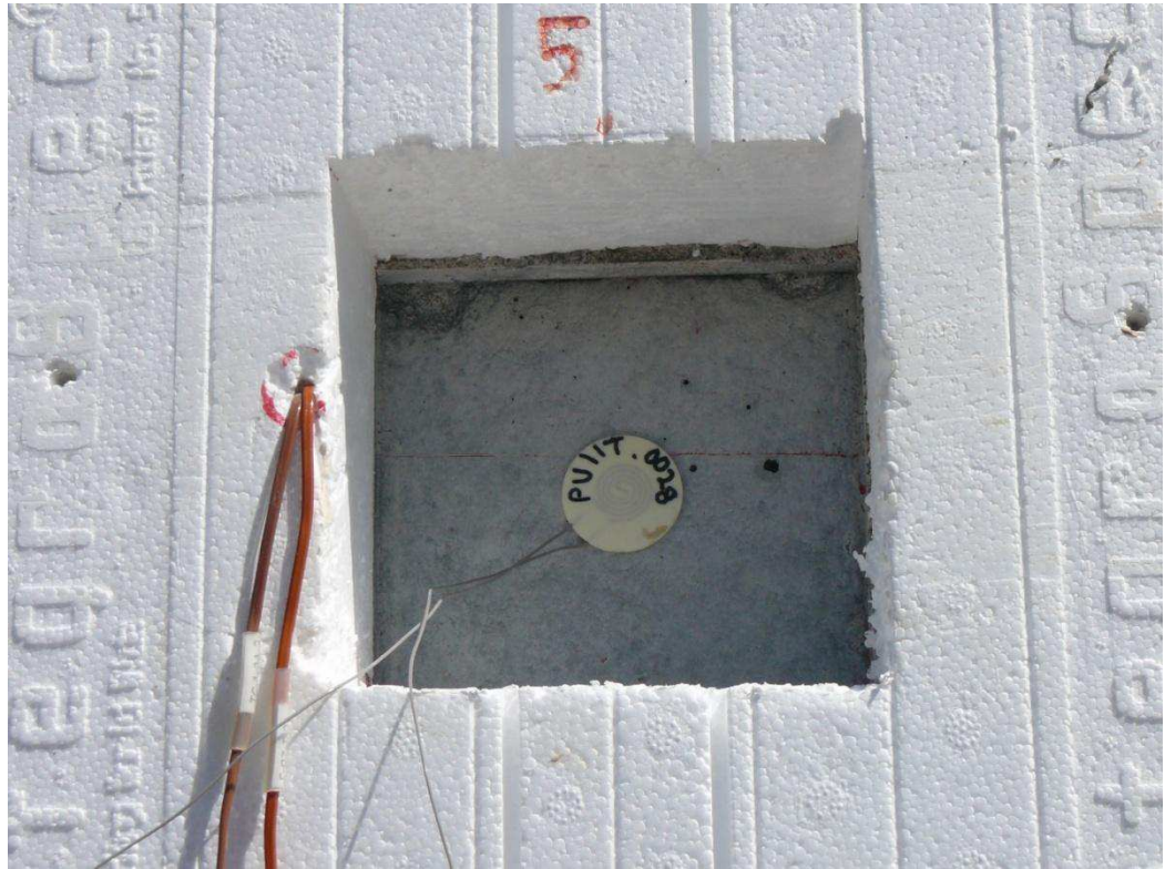
Figure A-62. Positioning of a heat flux transducer on the surface of the concrete.
