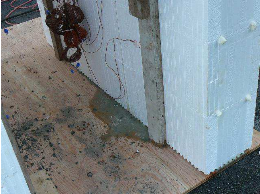
Figure A-13. Water pooling at the base of the ICF wall specimen after pouring the concrete.
