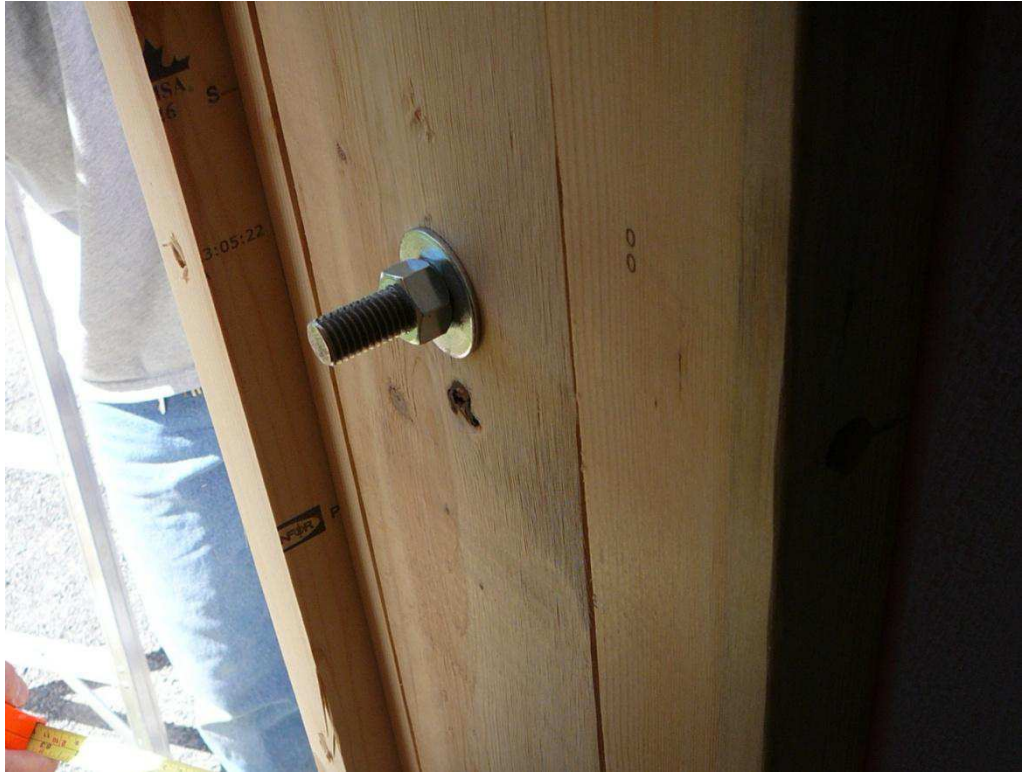
Figure A-32. Bolts secure the ICF wall specimen to the wood framing (2 bolts on each side).
