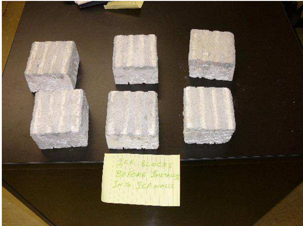
Figure A-60. The foam blocks with cured concrete, prior to installation into the ICF walls.
