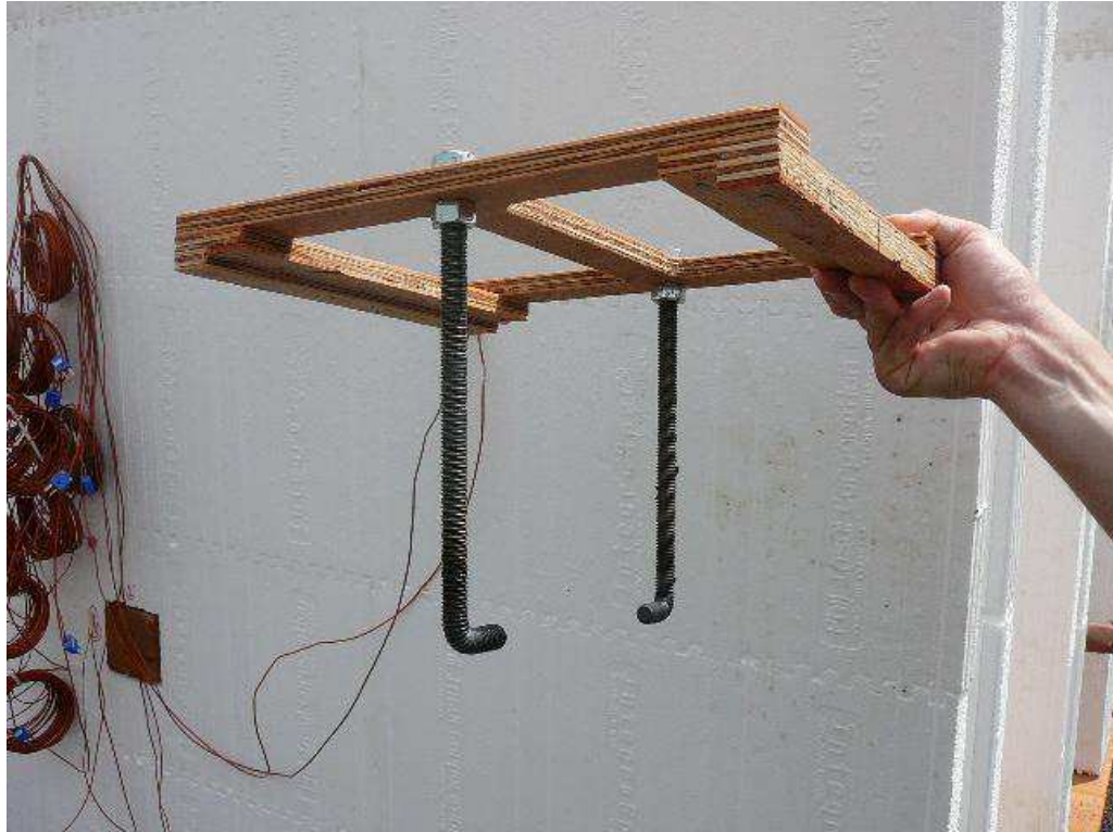
Figure A-15. Wooded alignment jig with threaded rods for the forklift lifting points.
