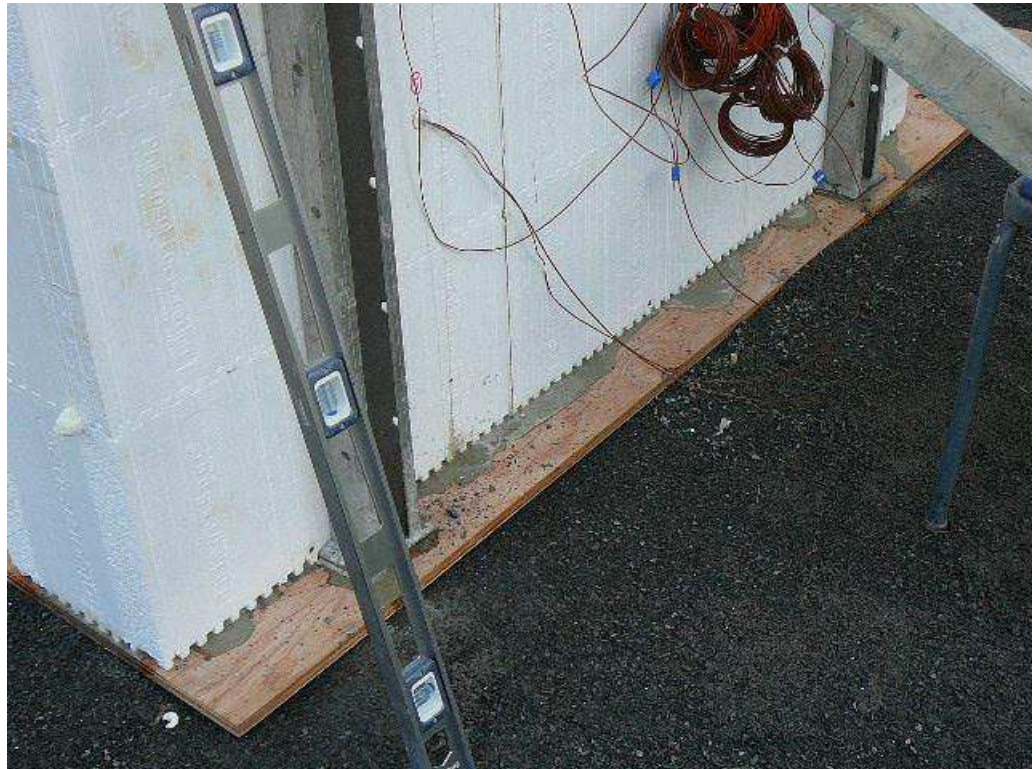
Figure A-14. Water pooling at the base of the ICF wall specimen after pouring the concrete.
