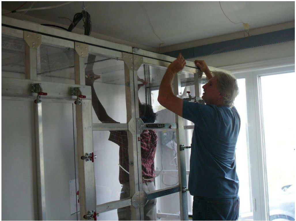
Figure A-53. Installation of the interior climate control chamber.
