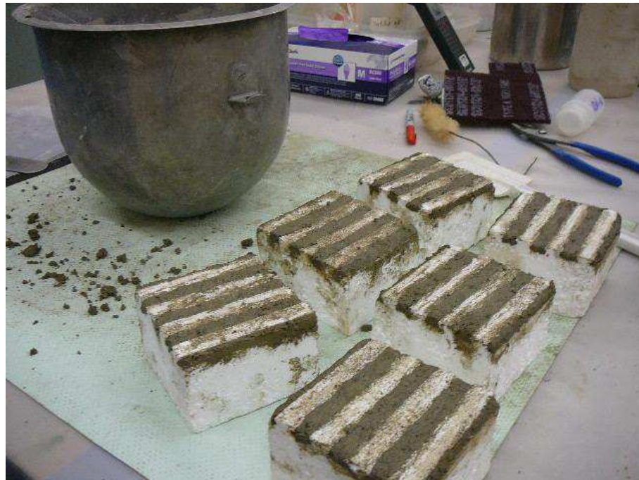
Figure A-57. Filling the ridges of the foam blocks with concrete.
