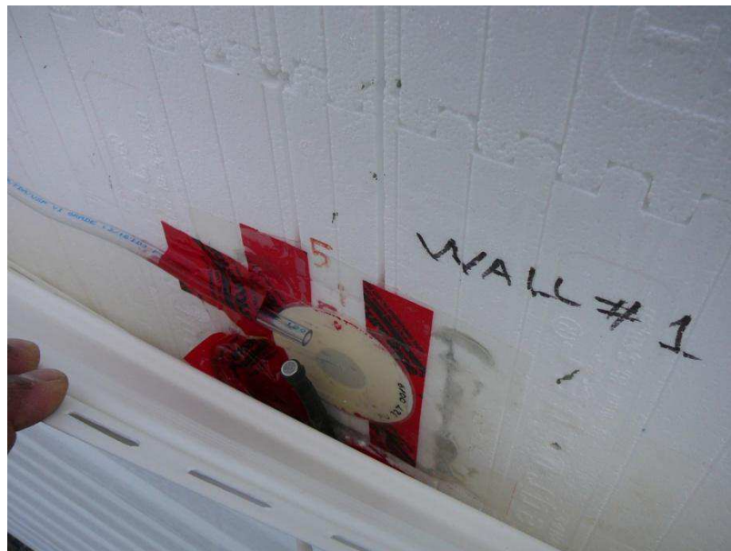
Figure A-40. Detail view of instrumentation behind the vinyl siding – including: a heat flux transducer (round disk), pressure tap (clear plastic tube), and RH&T sensor (black sensor).
