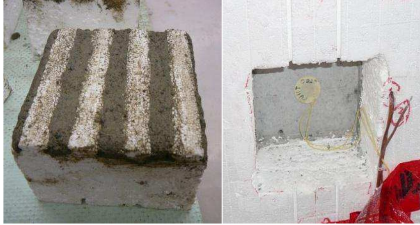
Figure 4. Removed section of EPS foam for heat flux transducer installation
