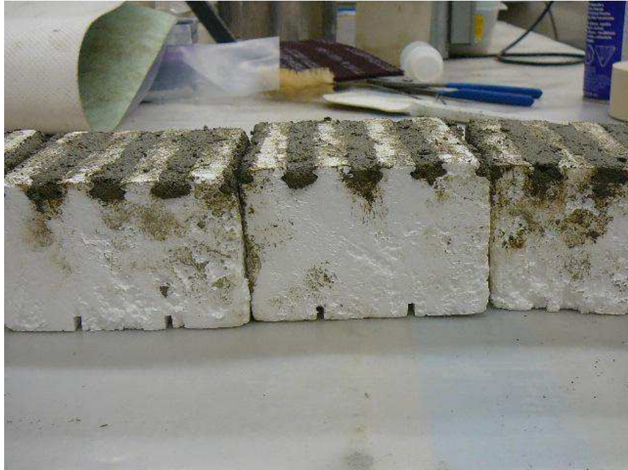
Figure A-58. Filling the ridges of the foam blocks with concrete.
