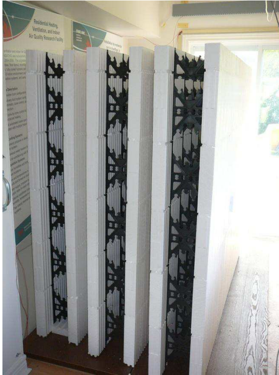
Figure A-4. Three assembled insulating forms inside the Research House. Note: three ICF wall specimens were fabricated, although only two were installed for monitoring at the FEWF. The third wall was made as a backup, in case either of the other two wall specimens was damaged during installation.
