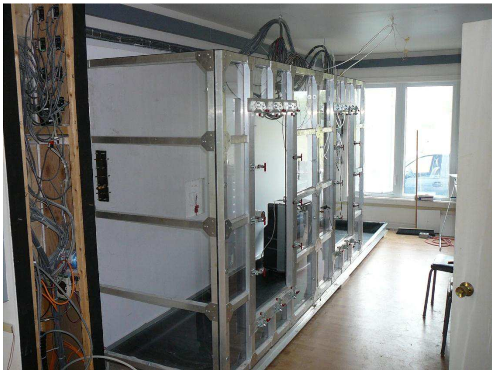
Figure A-52. Installation of the interior climate control chamber.
