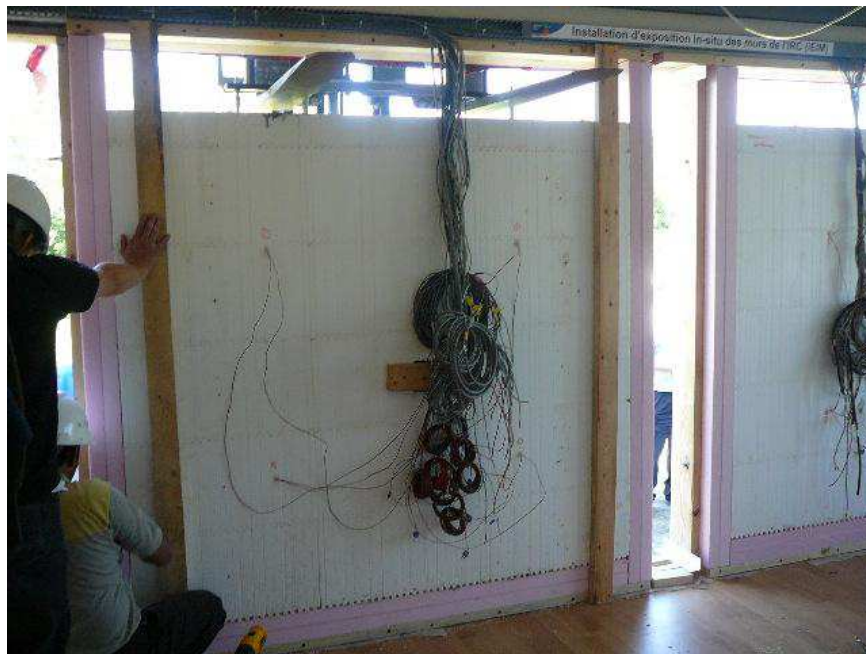
Figure A-27. Securing the second ICF wall specimen. Temporary vertical wood straps help guide the ICF wall specimen into place in the FEWF opening.
