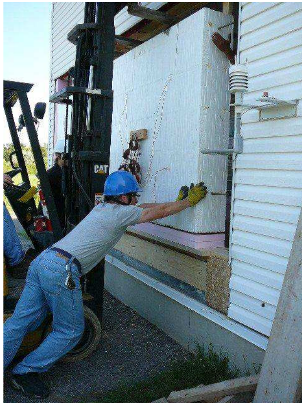
Figure A-25. Lifting the second ICF wall specimen into position.
