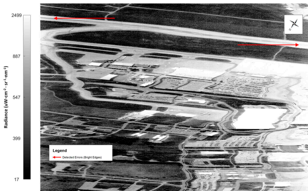
Figure 14. Histogram-equalized CASI image (24 June with the original processing) at 393.068 nm. The asphalt road along the south side of the image was brightest along the edge pixels. The errors in the data are highlighted by the red arrows.
