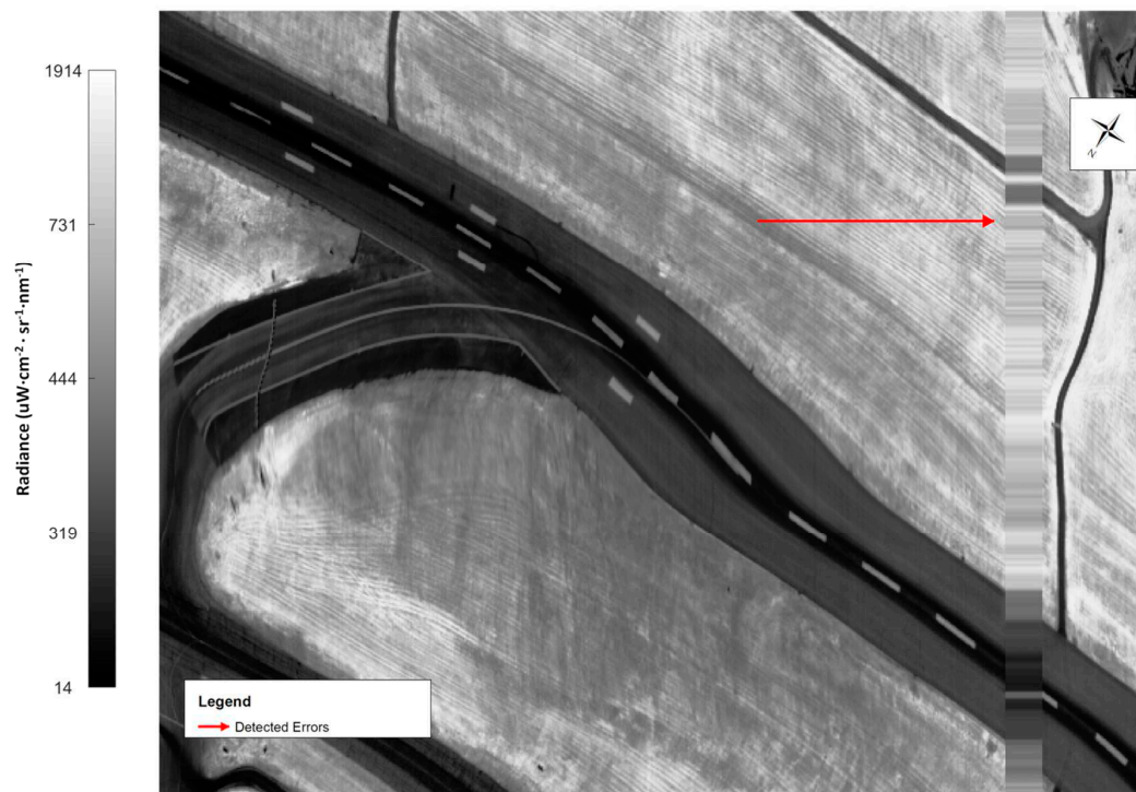
Figure 16. Histogram-equalized SASI imagery (24 June with the refined processing) at 1003 nm. An error across Pixels 548–564 is identified by the red arrow.
