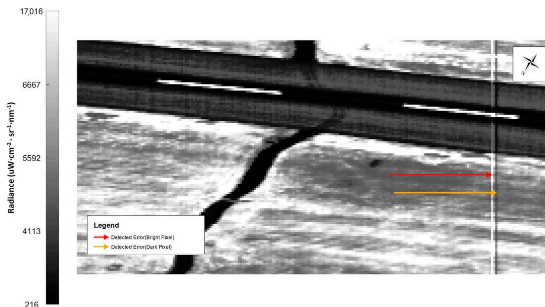
Figure 20. Histogram-equalized CASI (24 June with original processing) imagery at 744.653 nm. The image is zoomed in to display Columns 1248–1482 from left to right. The red and orange arrows point to the errors in Pixels 1454 and 1456 in the cross-track, respectively. These errors were visualized as a bright and dark vertical stripe.
