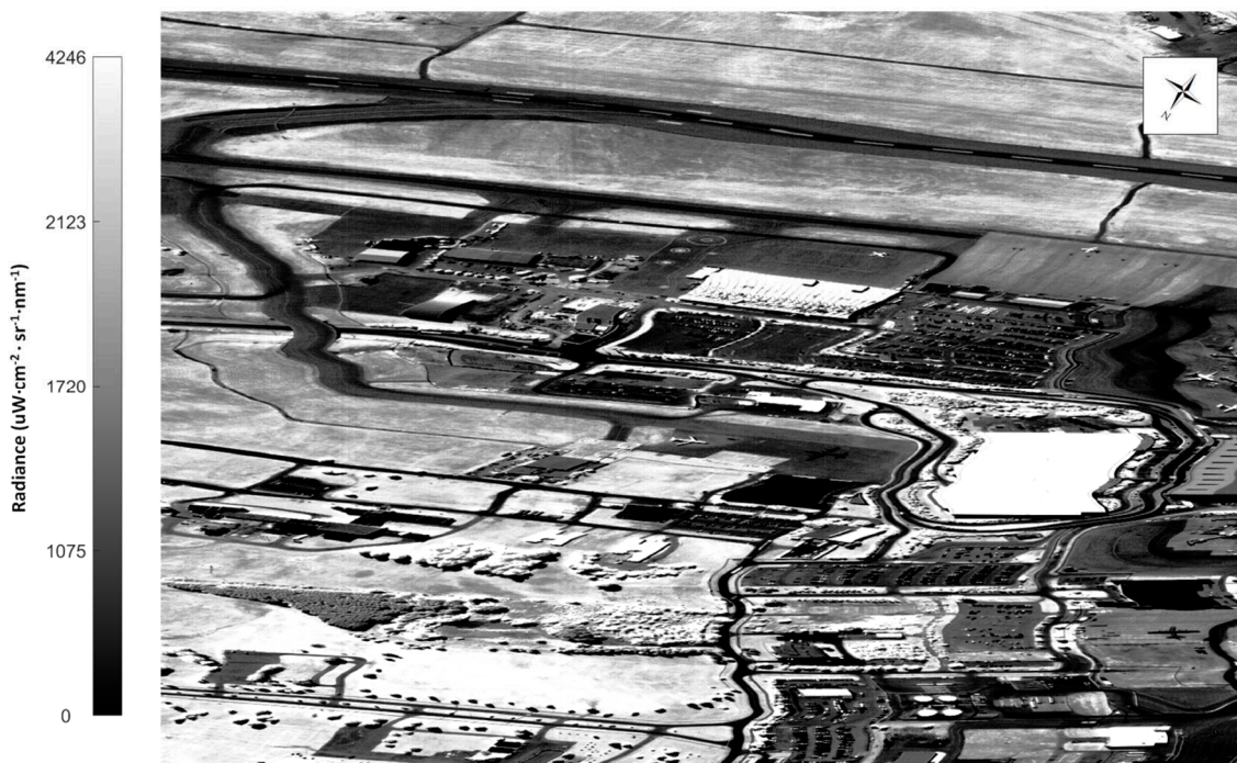
Figure 22. Histogram-equalized CASI imagery (24 June with original processing) at 931.099 nm. The imagery is stable, with no obvious errors.
