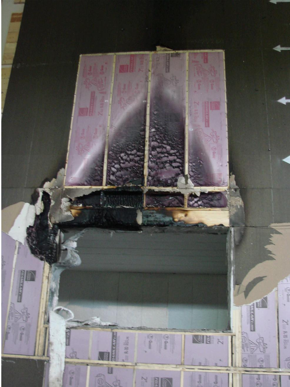
Figure 13. Wall Sample after Fire Exposure.
