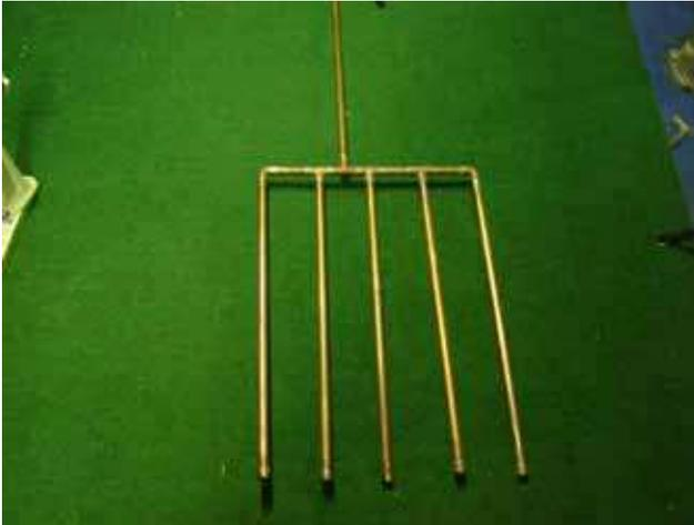
Figure 11, Five-fingered vertical seeding rake
