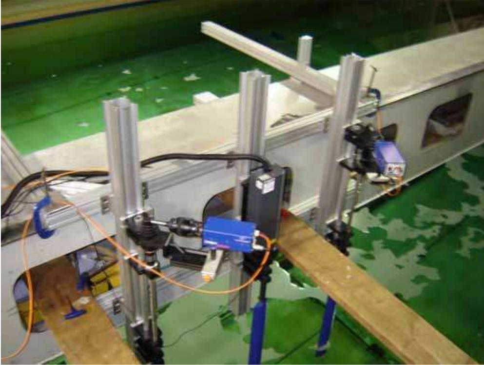
Figure 2, PIV system fitted to towing carriage
