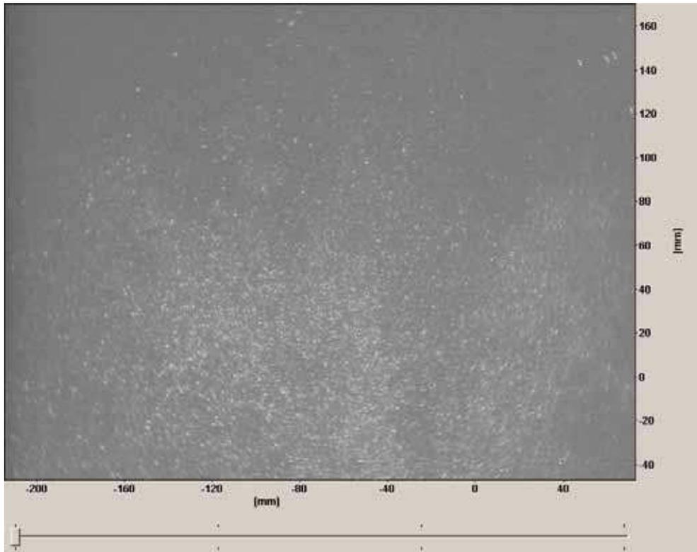
Figure 19, Particle distribution behind the seeding rake, 0.5 m/s
