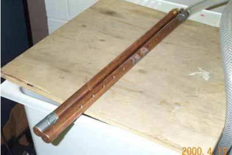
Figure 8, Prototype seeding rakes (rake with large diameter holes on right)
