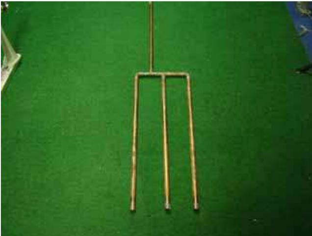
Figure 12, Three-fingered vertical seeding rake
