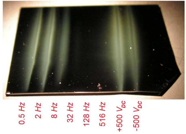
**Fig. 5.** Mechanism of droplet precipitation. Aerosol deposition performed under alternating voltage (500 V amplitude) at various frequencies (0.5–516 Hz) is compared with deposition at constant voltage. Concentration and duration were 2  $\mu\text{g}/\text{mL}$  and 90 s, respectively. Sample dimension is 25  $\times$  30  $\text{mm}^2$ , approximately.
