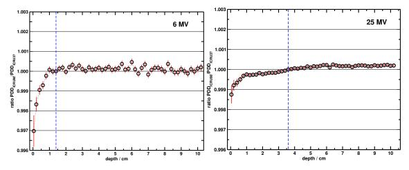
**FIGURE 1:** Ratios of Elekta Precise PDD curves for 6 MV and 25 MV photon beams for a 10 cm  $\times$  10 cm field and an SSD of 100 cm. The vertical dashed line indicates the position of the maximum dose, D<sub>max</sub>. The value at 10 cm depth can be used as an indicator for any relative variation in the beam quality specifier, % dd(10).
